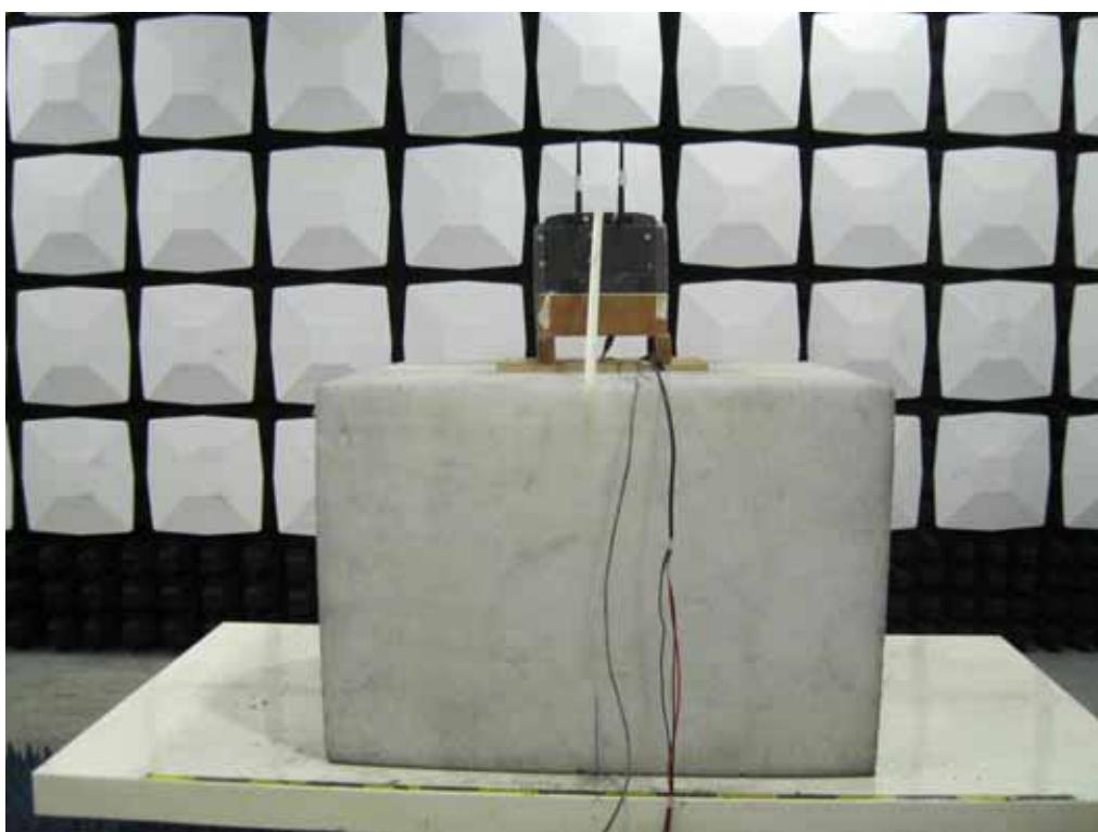
**ANTENNA PORT CONDUCTED RF MEASUREMENT SETUP**
