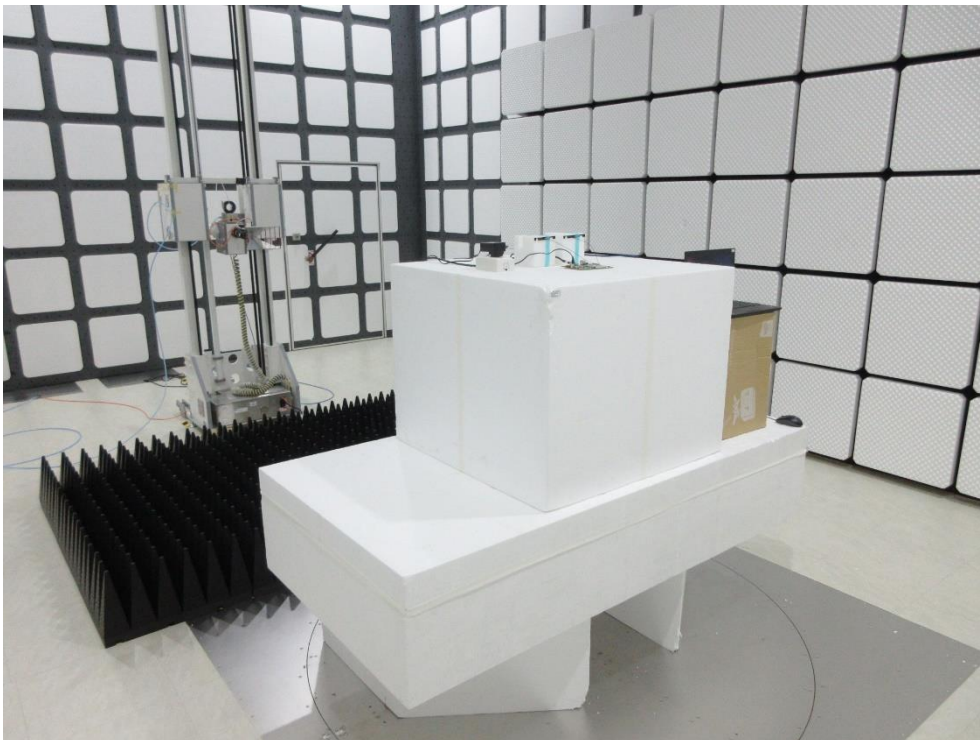
Description: Radiated Emission Test Setup for 1GHz~18GHz
