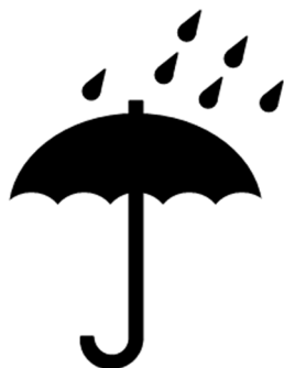
Figure 5: Safety marking "Keep dry"
