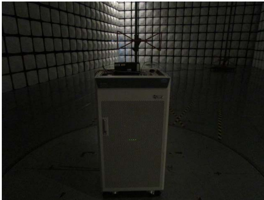
Transmitting Radiated Emissions Below 1 GHz– Front View (DC Source)
