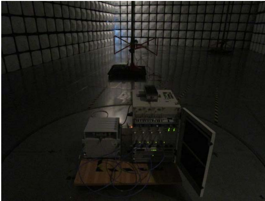
Transmitting Radiated Emissions Below 1 GHz– Front View (AC Source With Combiner)
