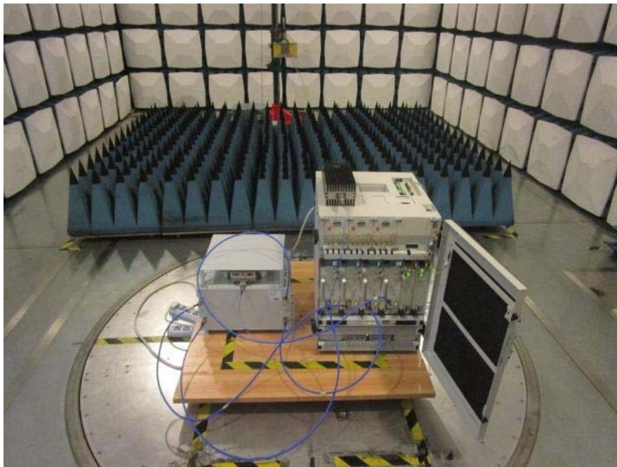
Transmitting Radiated Emissions Above 1 GHz– Front View (AC Source With Combiner)
