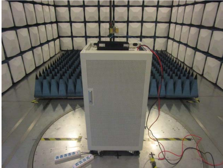
Transmitting Radiated Emissions Above 1 GHz– Rear View (DC Source)
