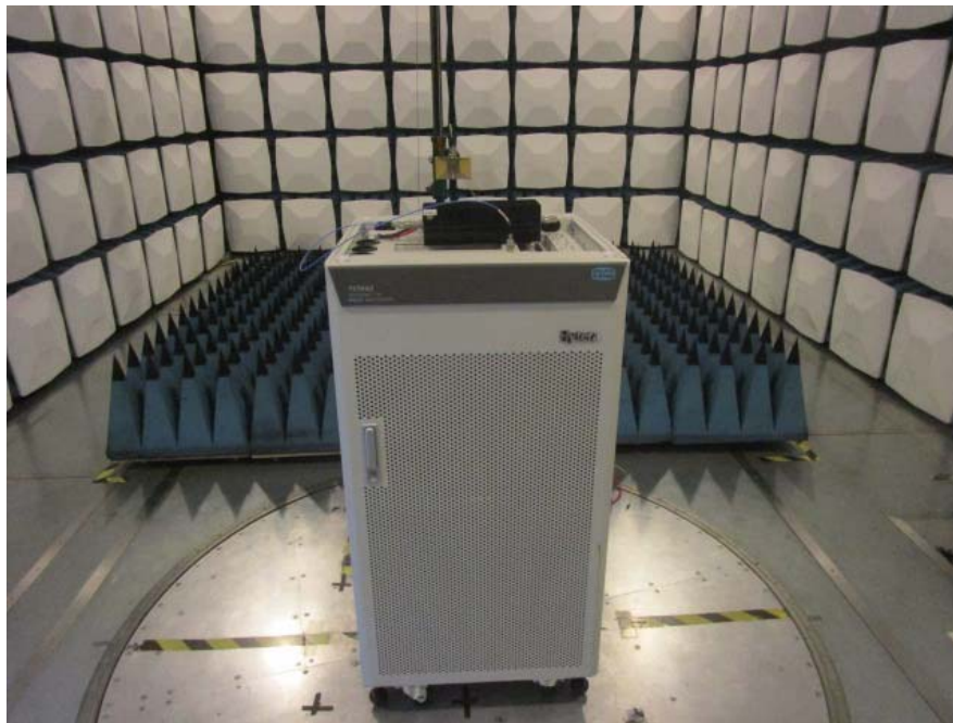
Transmitting Radiated Emissions Above 1 GHz– Front View (DC Source)
