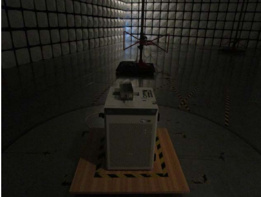
Transmitting Radiated Emissions Below 1 GHz– Front View (AC Source)
