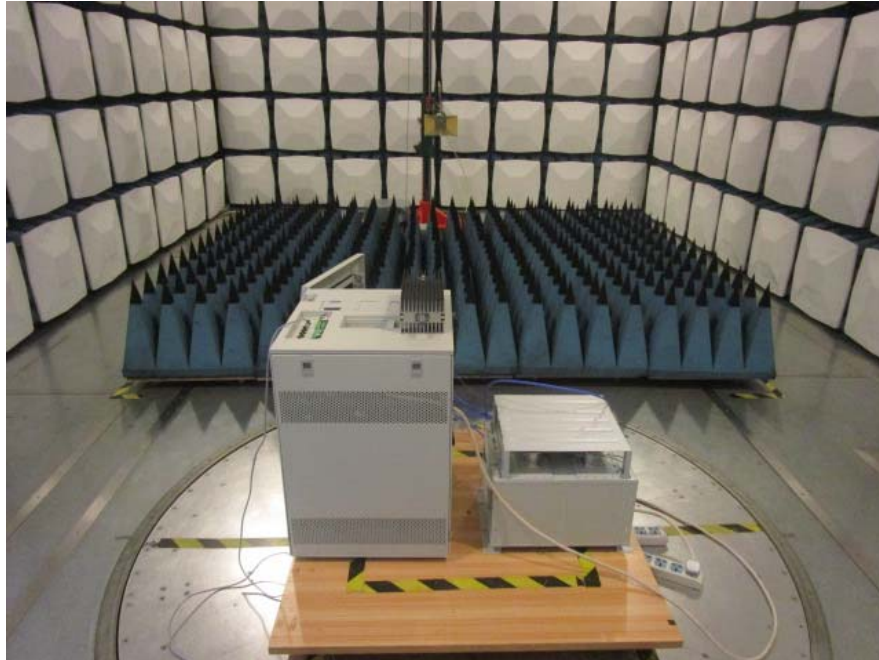
Transmitting Radiated Emissions Above 1 GHz– Rear View (AC Source With Combiner)
