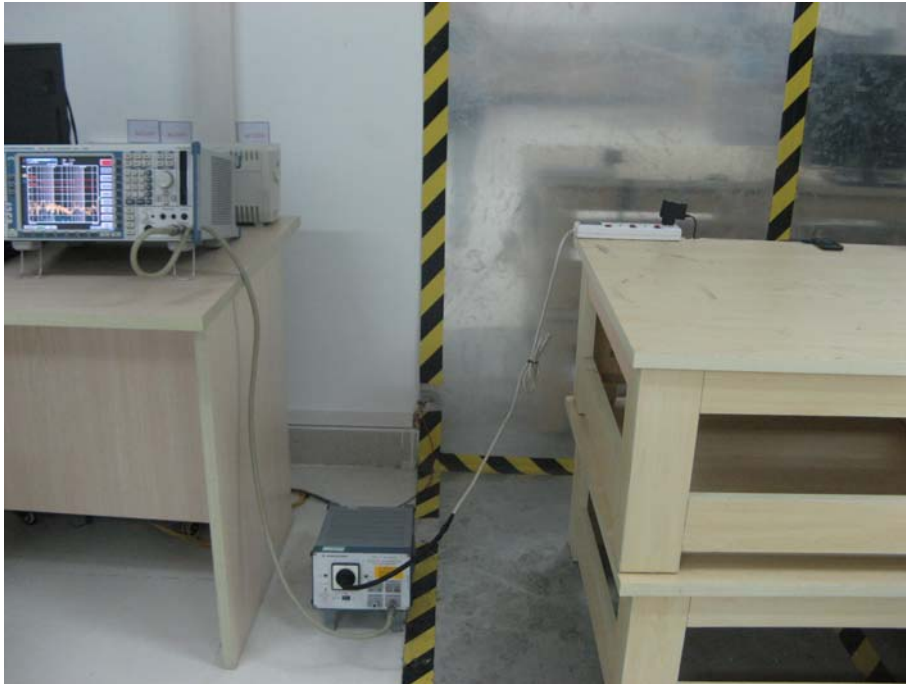
CONDUCTED EMISSION TEST SETUP
