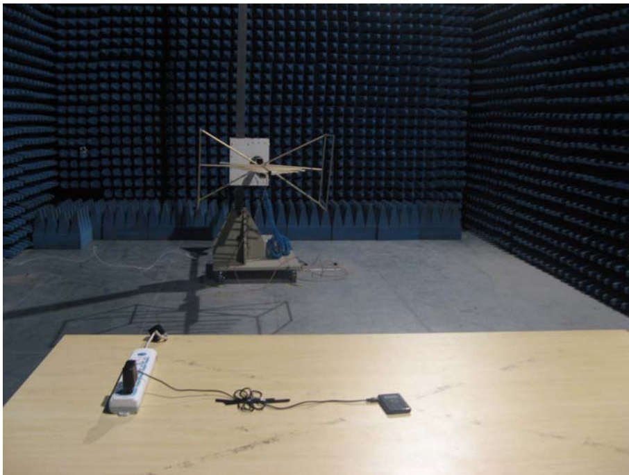
RADIATED EMISSION TEST SETUP
