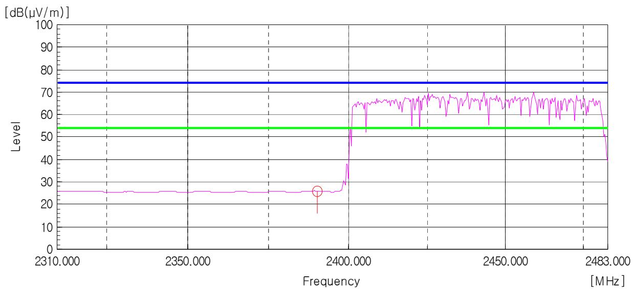
Peak Detector: RBW: 1 MHz, VBW: 1 MHz (2 483.5 MHz - 2 500.0 MHz), Worst case (High, Horizontal)
