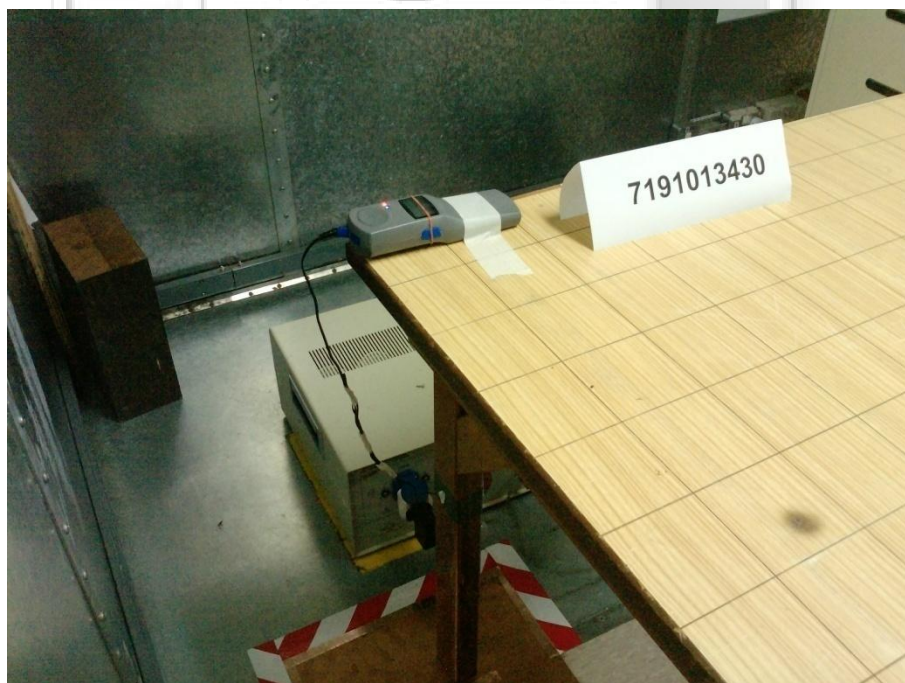
Conducted Emissions Test Setup (Rear View)
