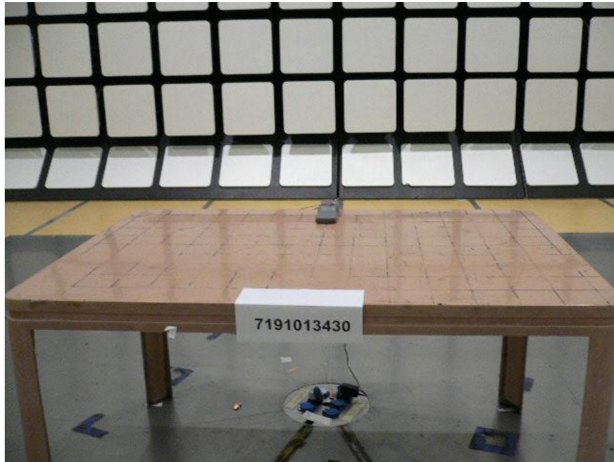
Radiated Emissions Test Setup (Front View)
