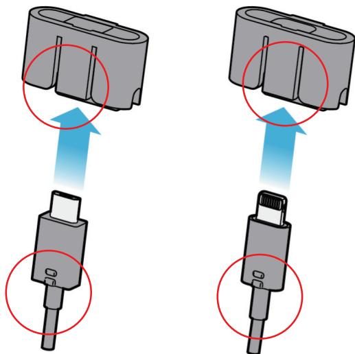
You can set up the cable height in two positions, depending on whether or not your smartphone is protected with a case. We recommend you to set the cable in its higher position if your smartphone is protected with a case.
