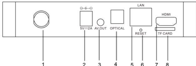
1. For External antenna    2. Power input    3. A/V out    4. OPTICAL
