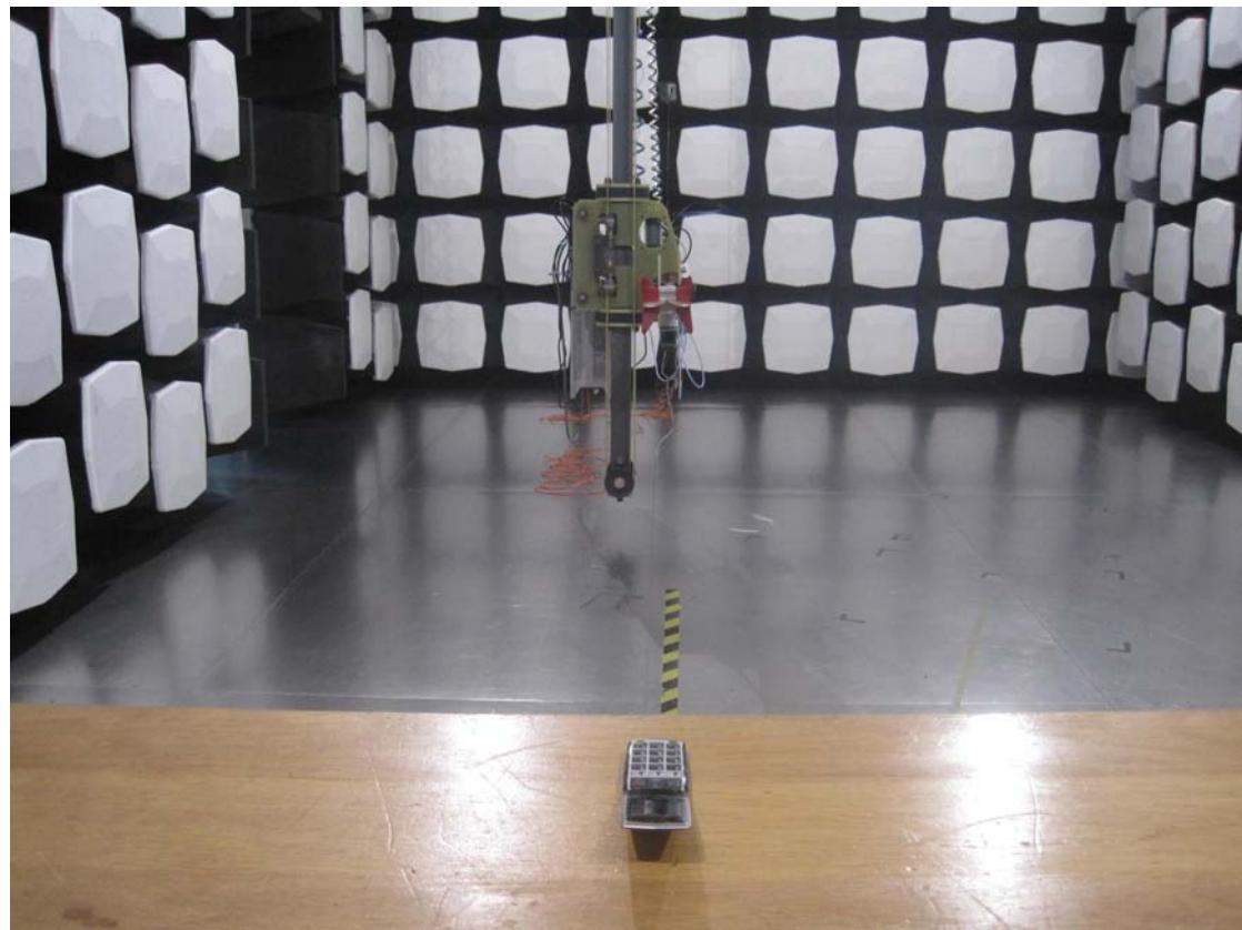
2. Part 15C Radiated emission above 1GHz
