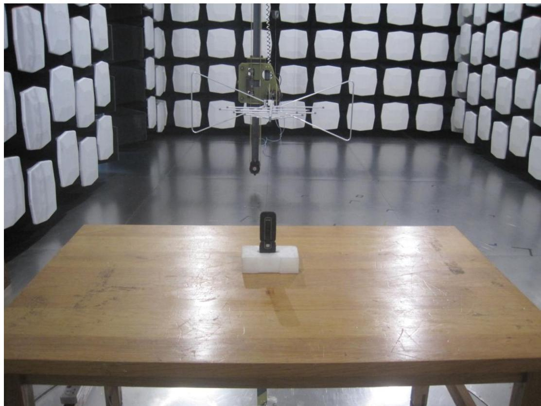
2. Part 15C Radiated emission above 1GHz
