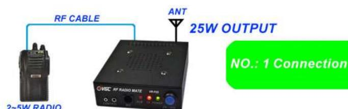
Option 2 : Only connect to the Antenna Jacks on the Radio and Amplifier – Use the accessory jack on the radio to an external mic or earpiece to operate the amplifier
