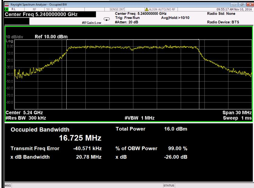
**IEEE 802.11a mode / 5260~ 5320MHz****26dB Bandwidth (CH Low)****Antenna 1**
