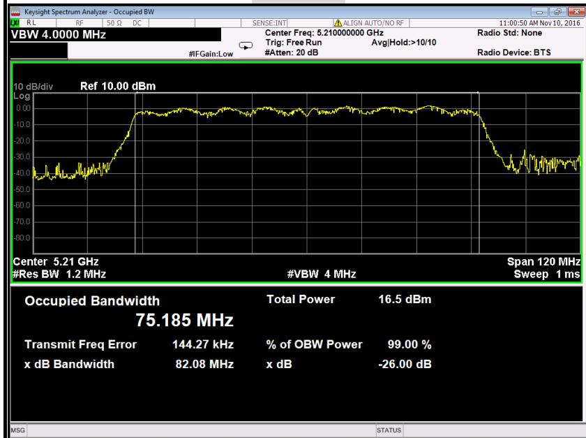
**IEEE 802.11ac 80 mode / 5290MHz****26dB Bandwidth****Antenna 0**
