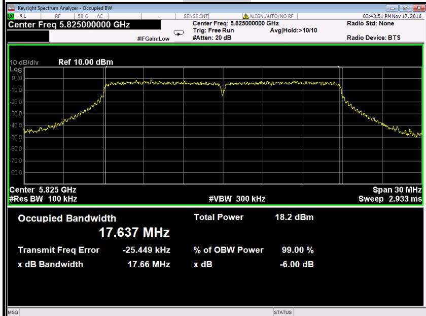
**IEEE 802.11n HT 20 MHz mode / 5745 ~ 5825MHz****6dB Bandwidth (CH Low)****Antenna 1**
