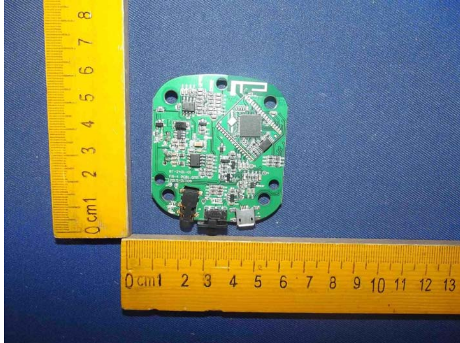
Figure 11 PCB of the EUT-Front View
