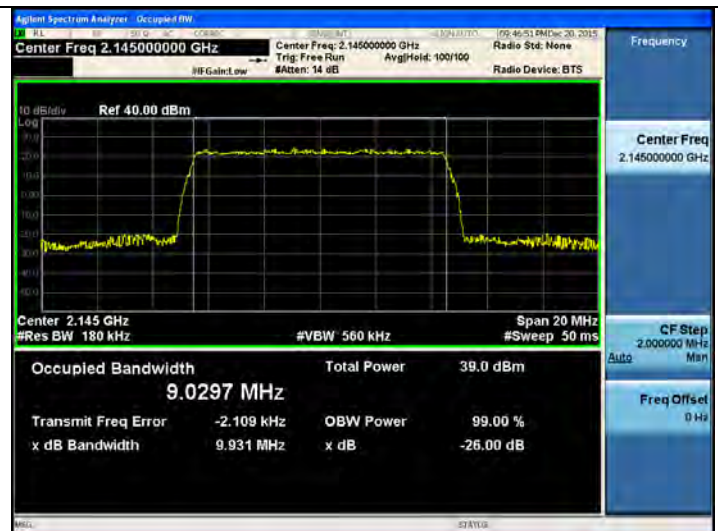
[AWS2100 AGC threshold Downlink Output LTE 10MHz Mid]
