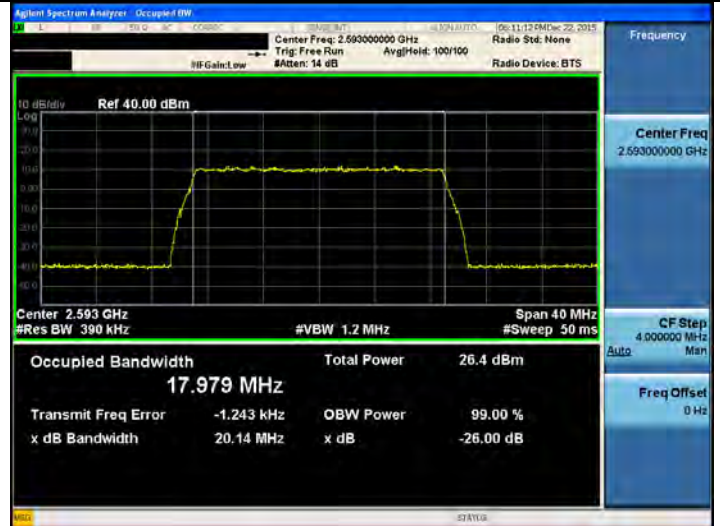
[BRS AGC threshold Downlink Input LTE10MHz Mid]
