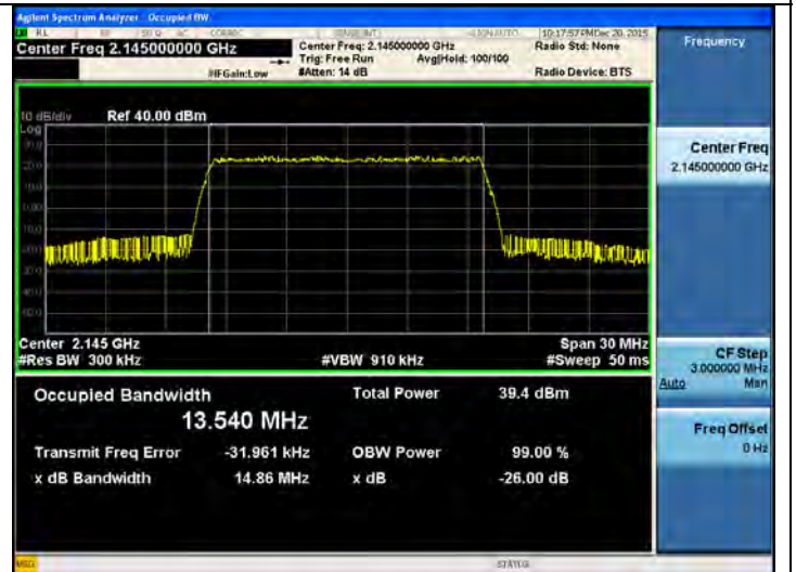
[AWS2100 AGC threshold Downlink Output LTE 15MHz Mid]
