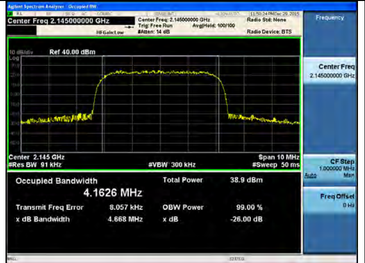
[AWS2100 AGC threshold Downlink Output UMTS Mid]
