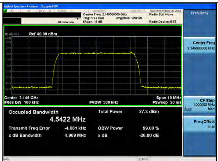
[AWS2100 AGC threshold Downlink Input LTE 5MHz Mid]
