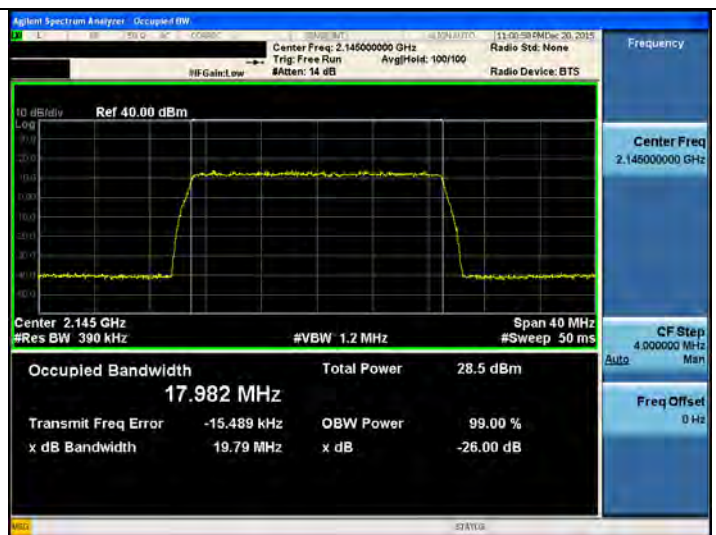
[AWS2100 AGC threshold Downlink Input LTE 20MHz Mid]
