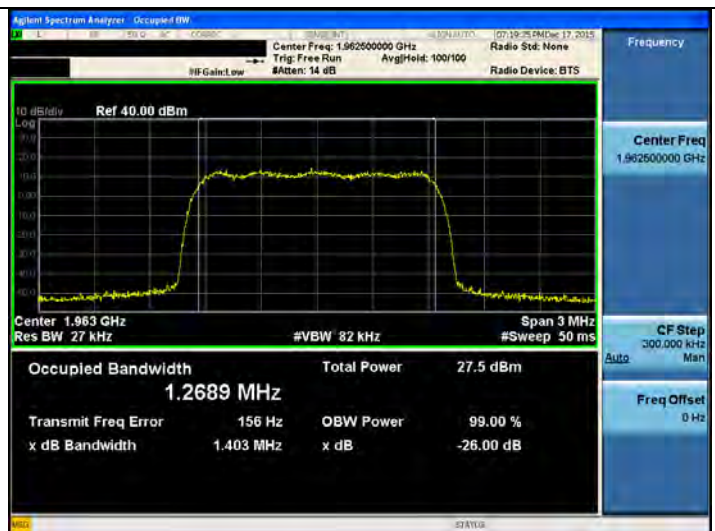
[PCS1900 AGC threshold Downlink Input CDMA Mid]
