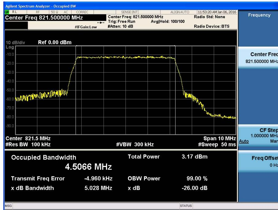
[800 Band +3 dB above the AGC threshold Uplink Output CDMA 1.25 MHz Low]
