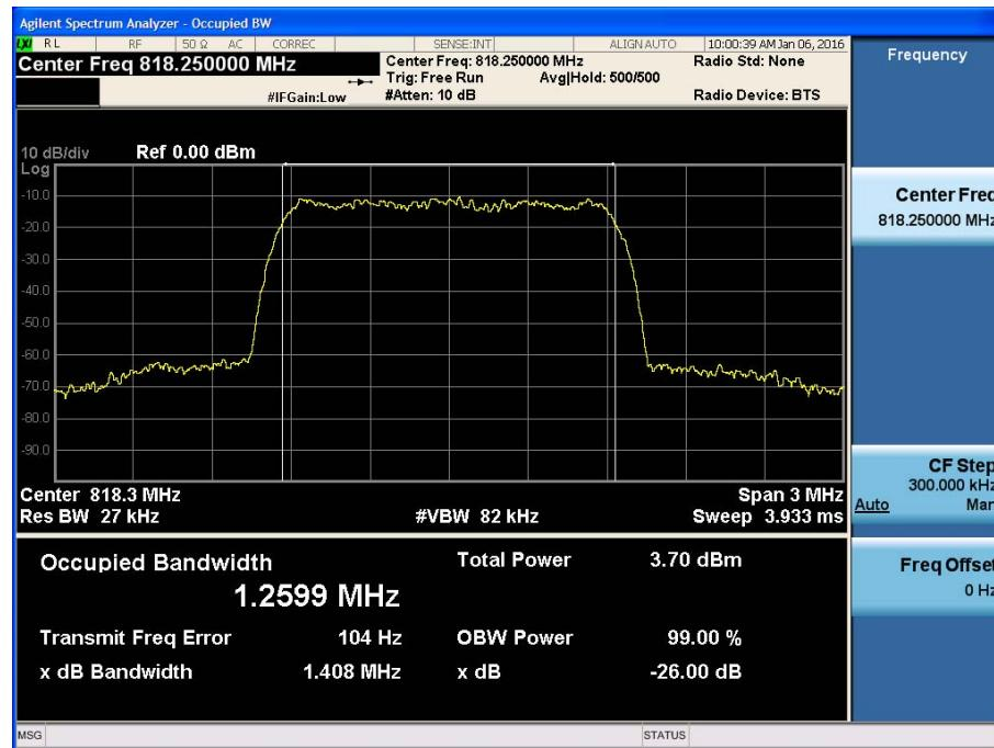
[800 Band +3 dB above the AGC threshold Uplink Output CDMA 1.25 MHz Middle]
