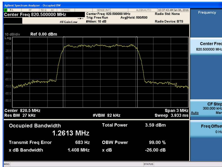
[800 Band +3 dB above the AGC threshold Uplink Output CDMA 1.25 MHz High]
