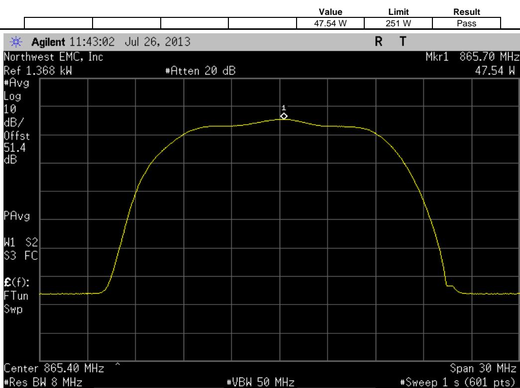
EVDO, Port B, Multi [3FA] Carrier, (862.9 MHz, 865.4 MHz, 867.9 MHz)
