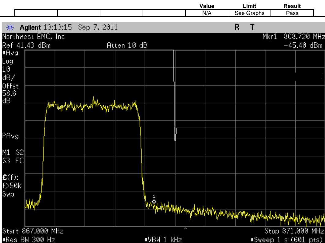
EVDO, Antenna Port A, Multi Carrier [5 FA], (862.9 MHz, 864.16 MHz, 865.4 MHz, 866.65 MHz, 867.9 MHz), Lower Band Edge Zoomed In
