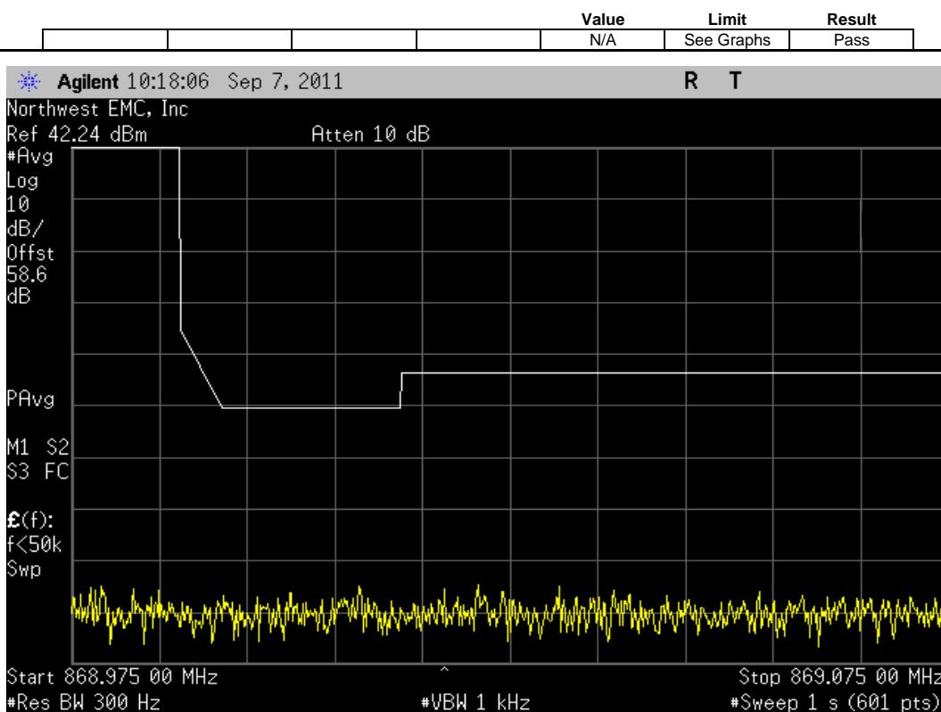
CDMA, Antenna Port A, Multi Carrier [3 FA], (862.9 MHz, 865.4 MHz, 867.9 MHz), Upper Band Edge Zoomed Out
