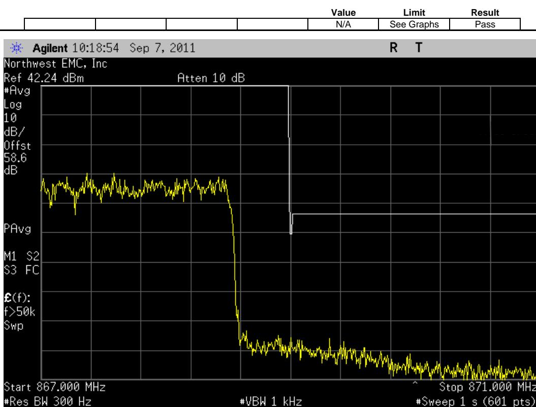
CDMA, Antenna Port A, Multi Carrier [5 FA], (862.9 MHz, 864.16 MHz, 865.4 MHz, 866.65 MHz, 867.9 MHz), Lower Band Edge Zoomed In
