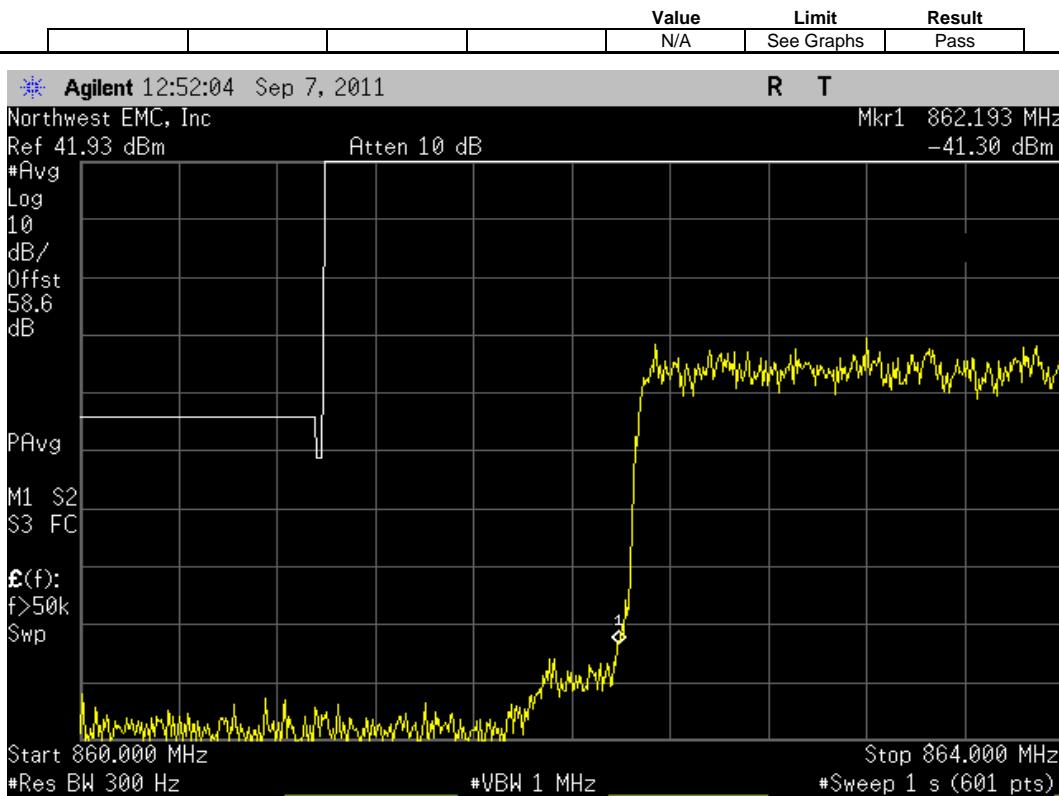
EVDO, Antenna Port B, Multi Carrier [5 FA], (862.9 MHz, 864.16 MHz, 865.4 MHz, 866.65 MHz, 867.9 MHz), Upper Band Edge Zoomed In
