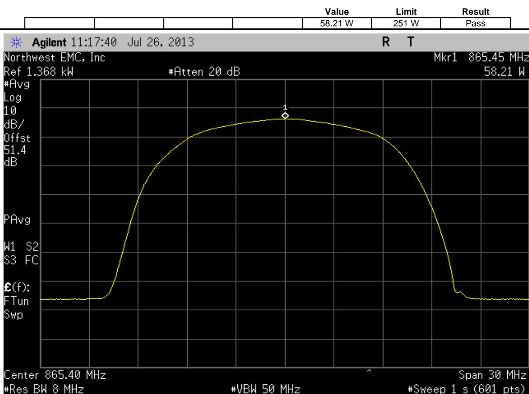
CDMA, Port B, Multi [5FA] Carrier, (862.9 MHz, 864.15, 865.4 MHz, 866.65, 867.9 MHz)
