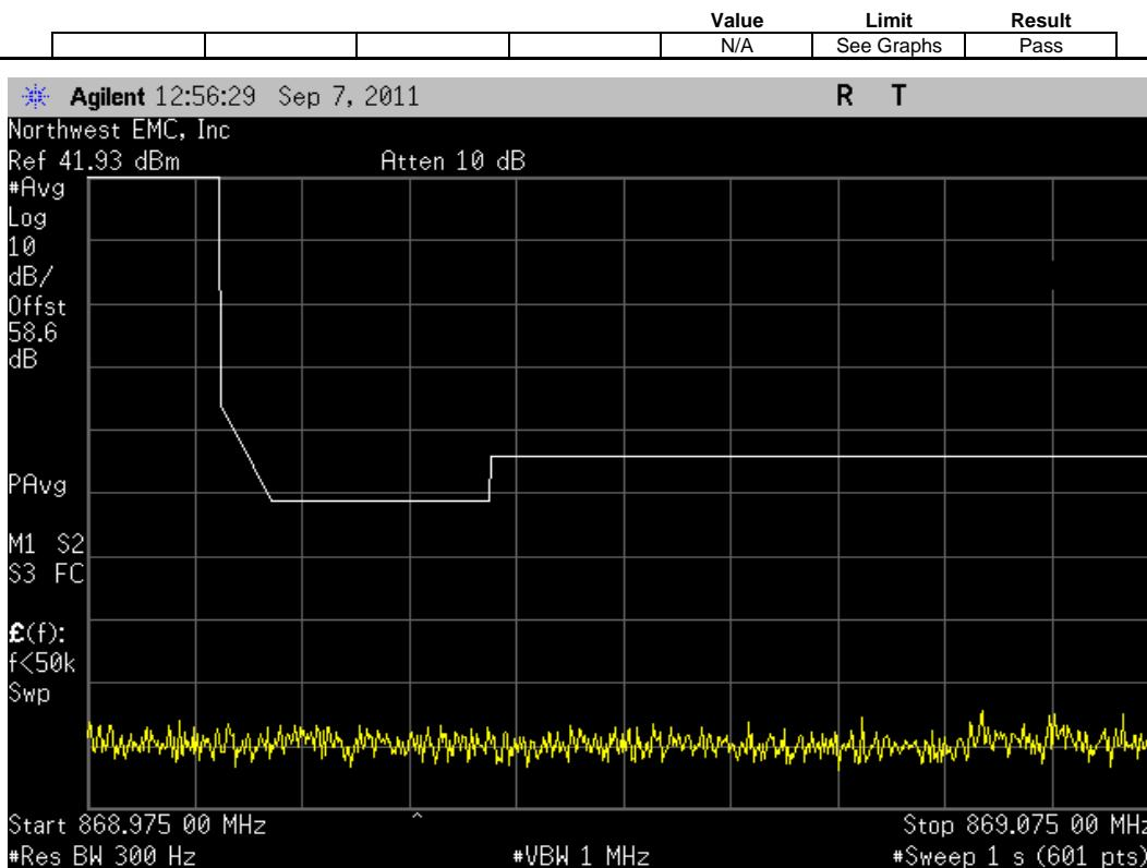
EVDO, Antenna Port B, Multi Carrier [5 FA], (862.9 MHz, 864.16 MHz, 865.4 MHz, 866.65 MHz, 867.9 MHz), Upper Band Edge Zoomed Out
