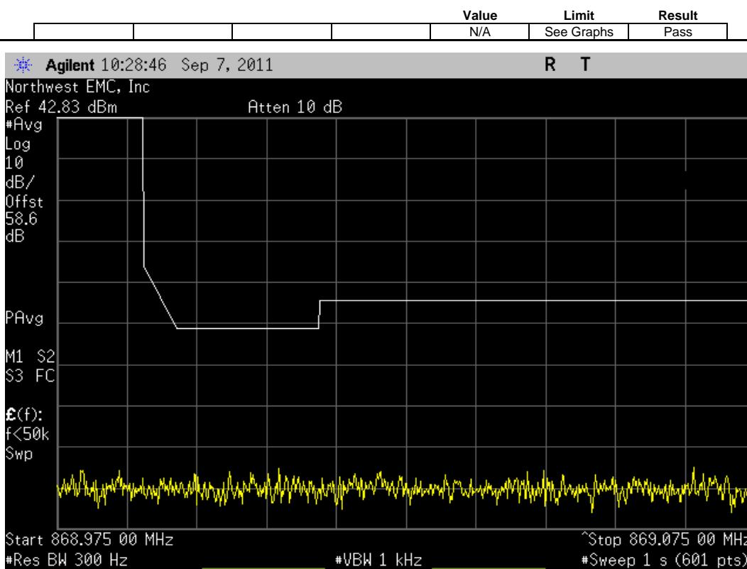
CDMA, Antenna Port A, Multi Carrier [5 FA], (862.9 MHz, 864.16 MHz, 865.4 MHz, 866.65 MHz, 867.9 MHz), Upper Band Edge Zoomed Out
