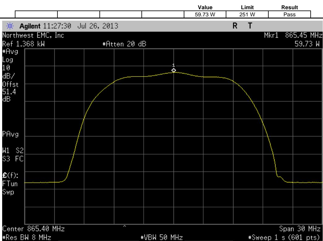
CDMA, Port B, Multi [3FA] Carrier, (862.9 MHz, 865.4 MHz, 867.9 MHz)
