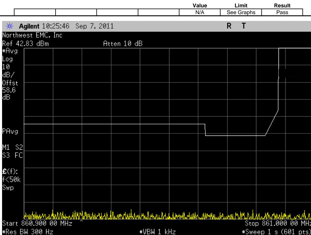
CDMA, Antenna Port A, Multi Carrier [5 FA], (862.9 MHz, 864.16 MHz, 865.4 MHz, 866.65 MHz, 867.9 MHz), Lower Band Edge Zoomed Out
