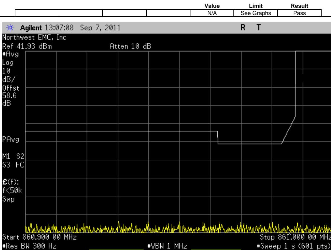
EVDO, Antenna Port A, Multi Carrier [5 FA], (862.9 MHz, 864.16 MHz, 865.4 MHz, 866.65 MHz, 867.9 MHz), Lower Band Edge Zoomed Out
