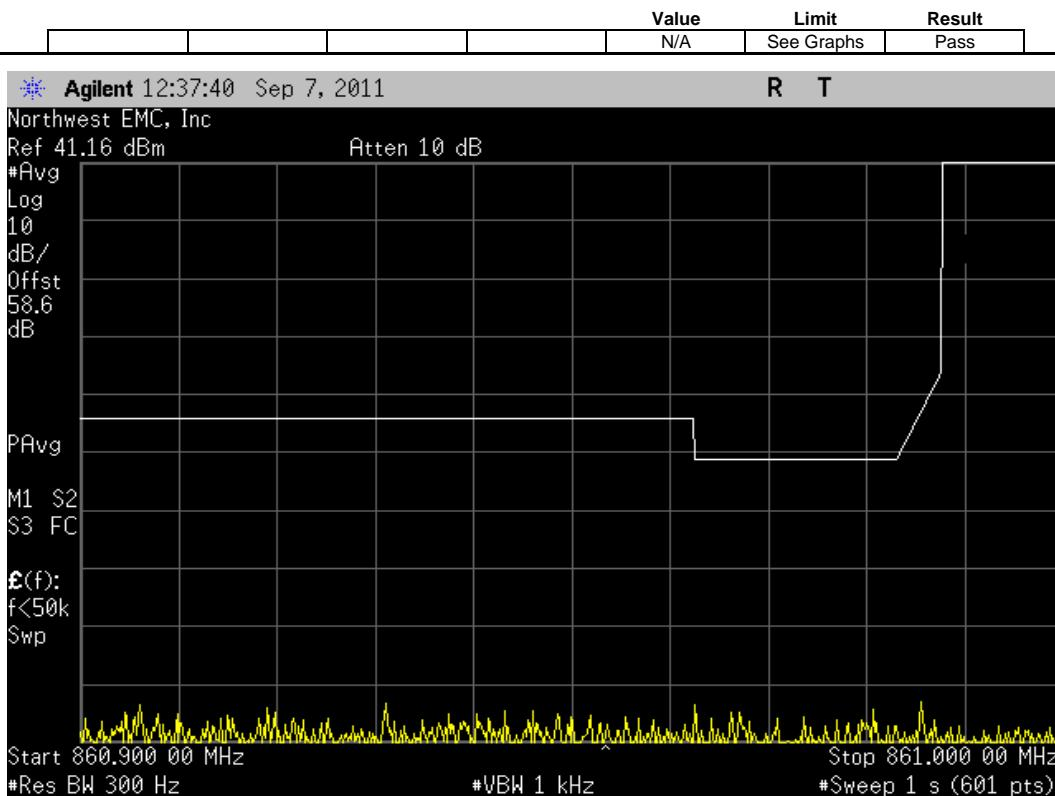
EVDO, Antenna Port B, Multi Carrier [3 FA], (862.9 MHz, 865.4 MHz, 867.9 MHz), Lower Band Edge Zoomed Out
