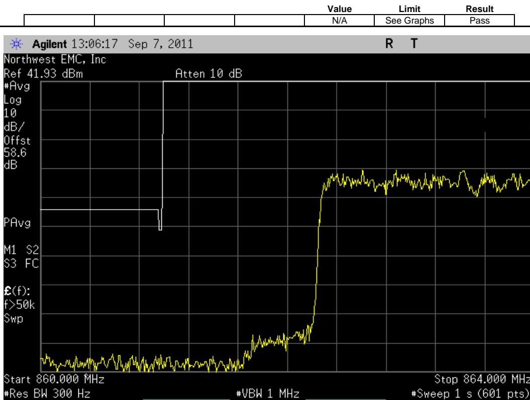
EVDO, Antenna Port A, Multi Carrier [5 FA], (862.9 MHz, 864.16 MHz, 865.4 MHz, 866.65 MHz, 867.9 MHz), Upper Band Edge Zoomed In
