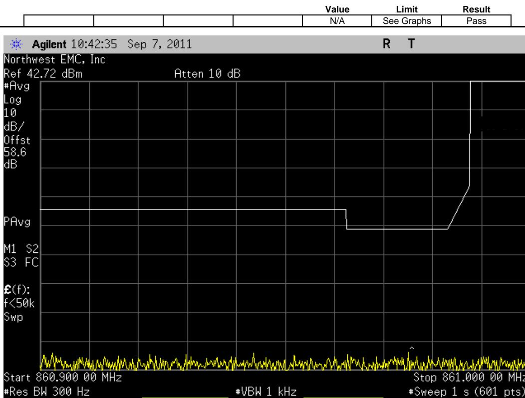
CDMA, Antenna Port B, Multi Carrier [5 FA], (862.9 MHz, 864.16 MHz, 865.4 MHz, 866.65 MHz, 867.9 MHz), Lower Band Edge Zoomed Out
