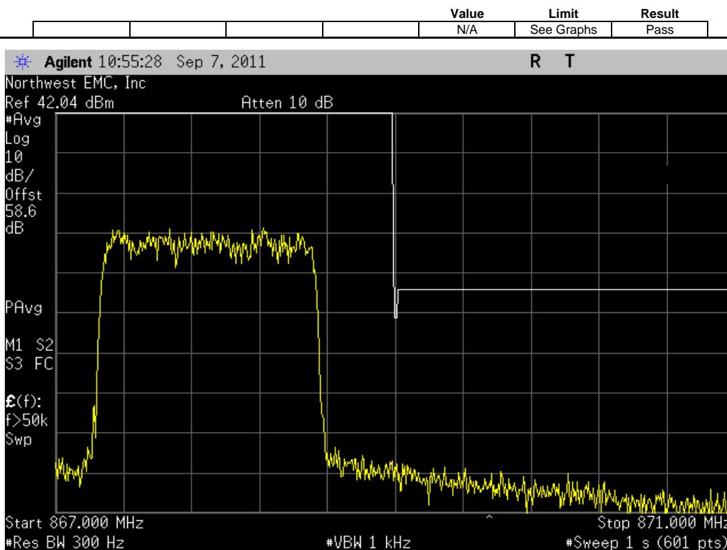
CDMA, Antenna Port B, Multi Carrier [5 FA], (862.9 MHz, 864.16 MHz, 865.4 MHz, 866.65 MHz, 867.9 MHz), Lower Band Edge Zoomed In
