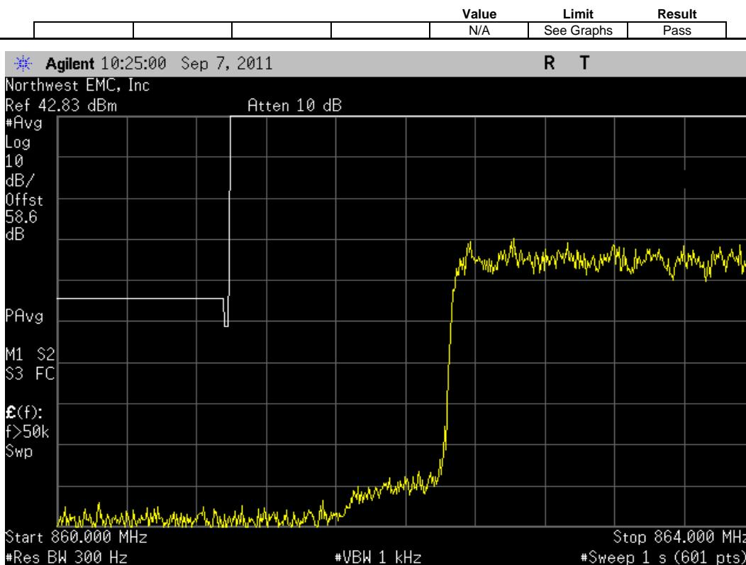
CDMA, Antenna Port A, Multi Carrier [5 FA], (862.9 MHz, 864.16 MHz, 865.4 MHz, 866.65 MHz, 867.9 MHz), Upper Band Edge Zoomed In
