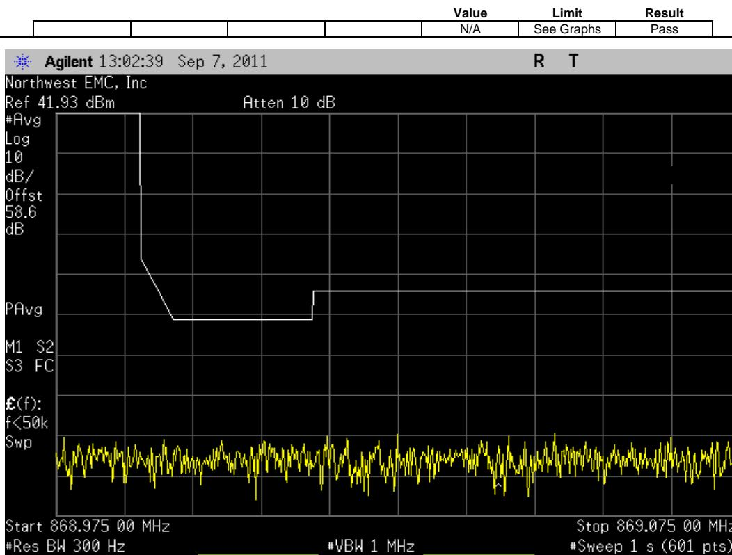
EVDO, Antenna Port A, Multi Carrier [5 FA], (862.9 MHz, 864.16 MHz, 865.4 MHz, 866.65 MHz, 867.9 MHz), Upper Band Edge Zoomed Out
