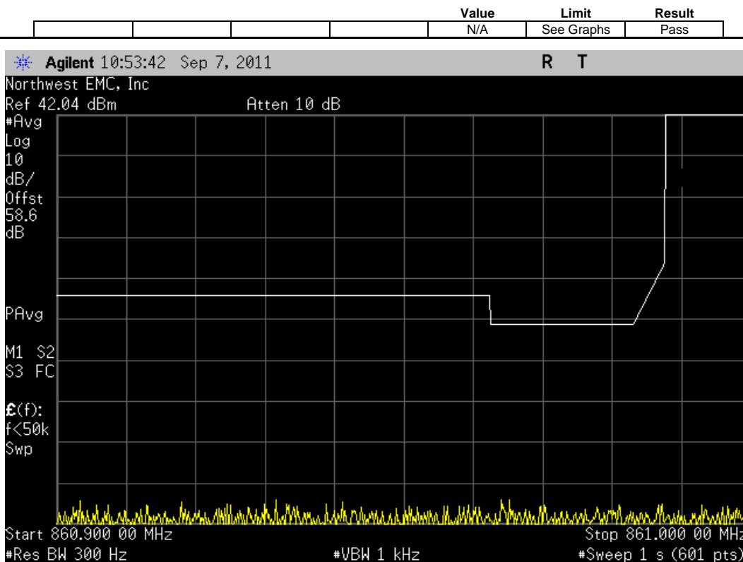
CDMA, Antenna Port B, Multi Carrier [3 FA], (862.9 MHz, 865.4 MHz, 867.9 MHz), Lower Band Edge Zoomed Out
