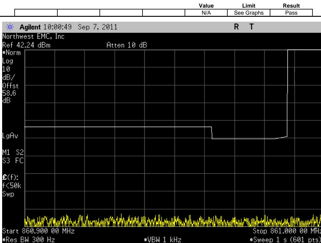
CDMA, Antenna Port A, Multi Carrier [3 FA], (862.9 MHz, 865.4 MHz, 867.9 MHz), Lower Band Edge Zoomed Out
