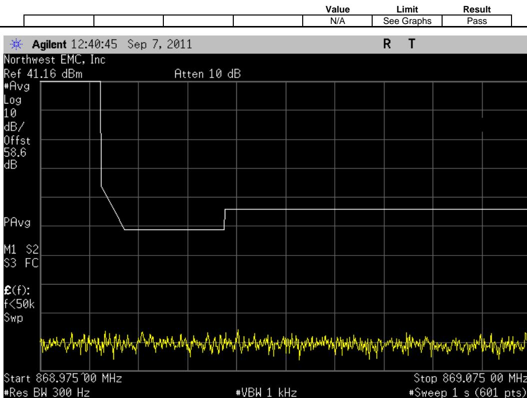
EVDO, Antenna Port B, Multi Carrier [3 FA], (862.9 MHz, 865.4 MHz, 867.9 MHz), Upper Band Edge Zoomed Out
