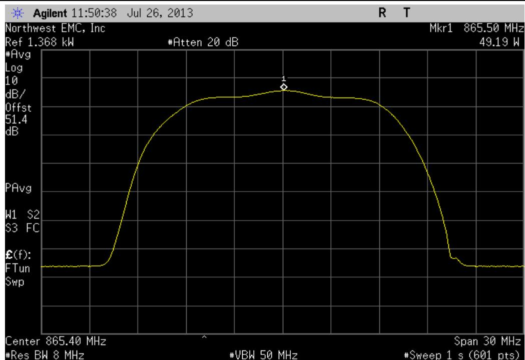
EVDO, Port A, Multi [3FA] Carrier, (862.9 MHz, 865.4 MHz, 867.9 MHz)
