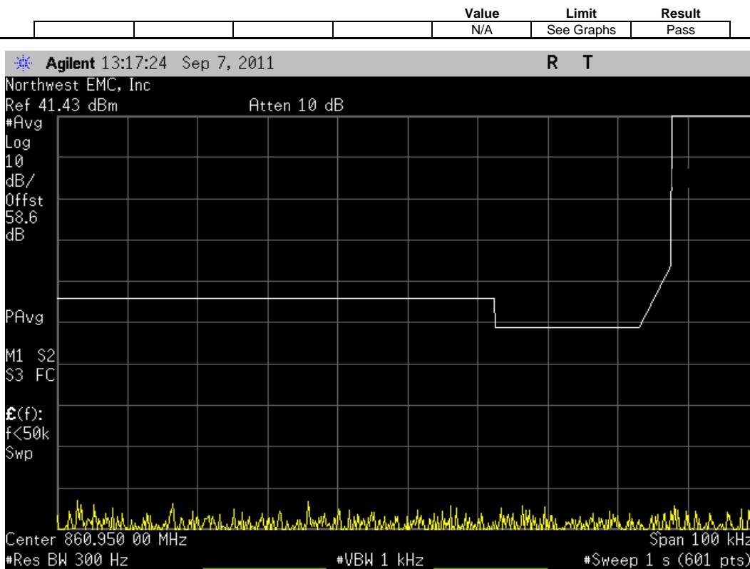
EVDO, Antenna Port A, Multi Carrier [3 FA], (862.9 MHz, 865.4 MHz, 867.9 MHz), Lower Band Edge Zoomed Out
