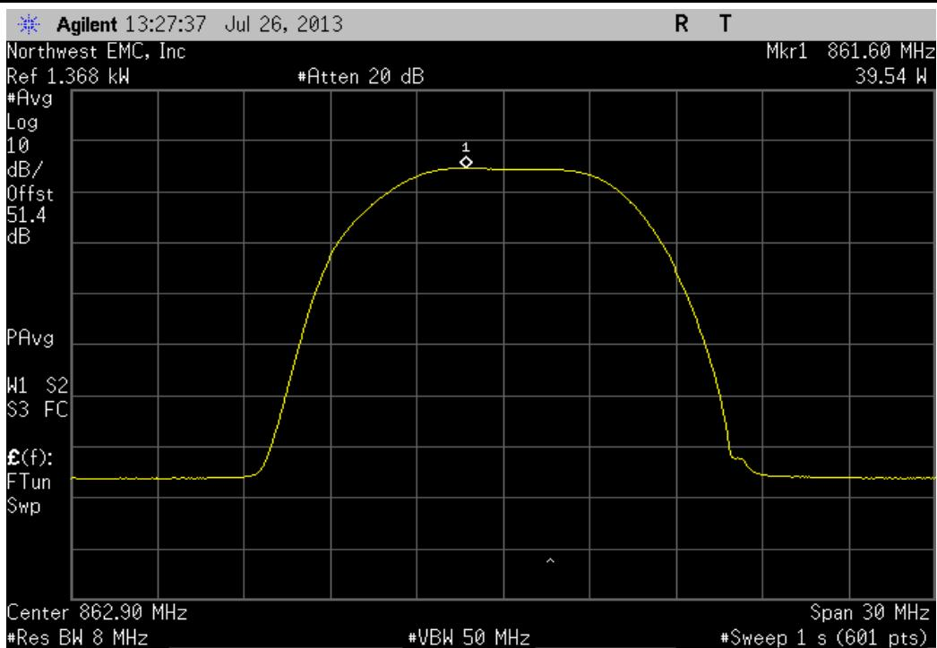
EVDO, Port B, Single Carrier, High Channel, 867.9 MHz
