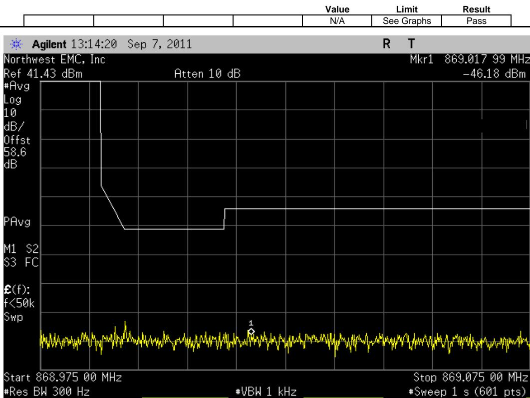
EVDO, Antenna Port A, Multi Carrier [3 FA], (862.9 MHz, 865.4 MHz, 867.9 MHz), Upper Band Edge Zoomed Out
