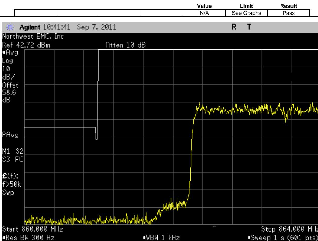
CDMA, Antenna Port B, Multi Carrier [5 FA], (862.9 MHz, 864.16 MHz, 865.4 MHz, 866.65 MHz, 867.9 MHz), Upper Band Edge Zoomed In
