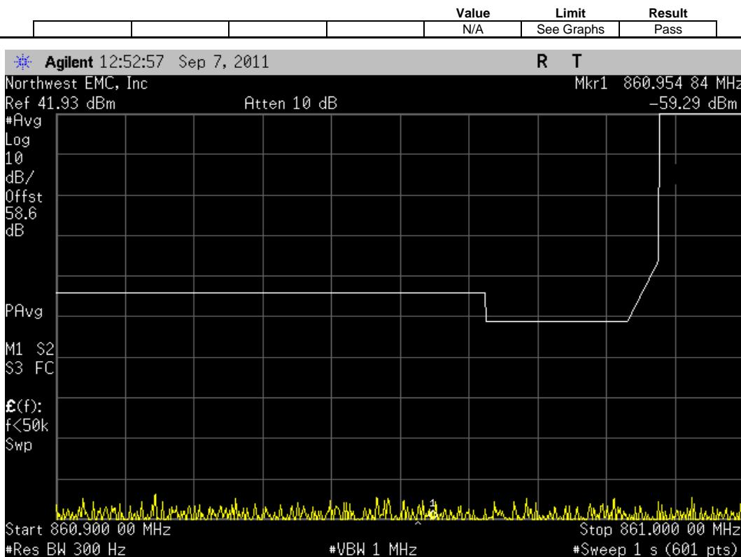
EVDO, Antenna Port B, Multi Carrier [5 FA], (862.9 MHz, 864.16 MHz, 865.4 MHz, 866.65 MHz, 867.9 MHz), Lower Band Edge Zoomed Out
