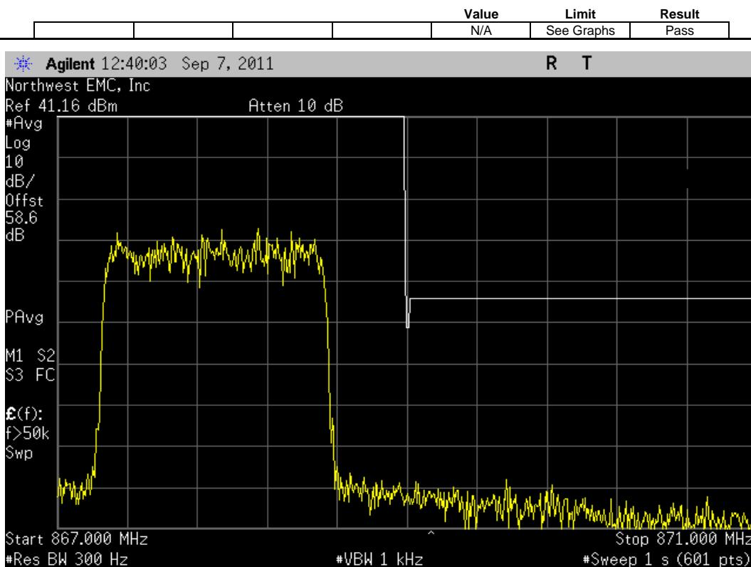
EVDO, Antenna Port B, Multi Carrier [5 FA], (862.9 MHz, 864.16 MHz, 865.4 MHz, 866.65 MHz, 867.9 MHz), Lower Band Edge Zoomed In
