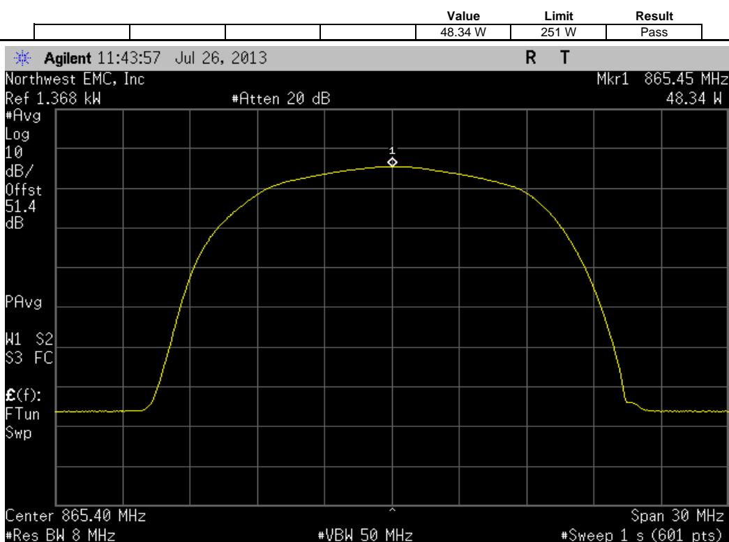
EVDO, Port B, Multi [5FA] Carrier, (862.9 MHz, 864.15, 865.4 MHz, 866.65, 867.9 MHz)
