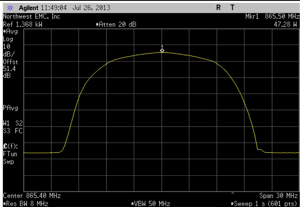
EVDO, Port A, Multi [5FA] Carrier, (862.9 MHz, 864.15, 865.4 MHz, 866.65, 867.9 MHz)
