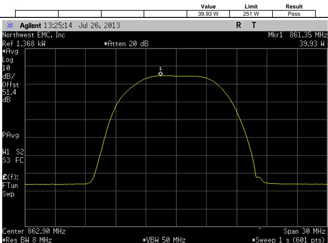
EVDO, Port A, Single Carrier, High Channel, 867.9 MHz
