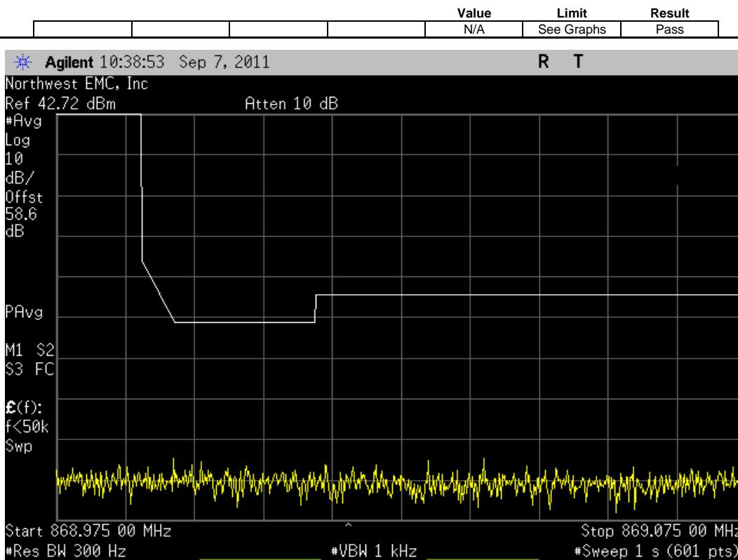
CDMA, Antenna Port B, Multi Carrier [5 FA], (862.9 MHz, 864.16 MHz, 865.4 MHz, 866.65 MHz, 867.9 MHz), Upper Band Edge Zoomed Out
