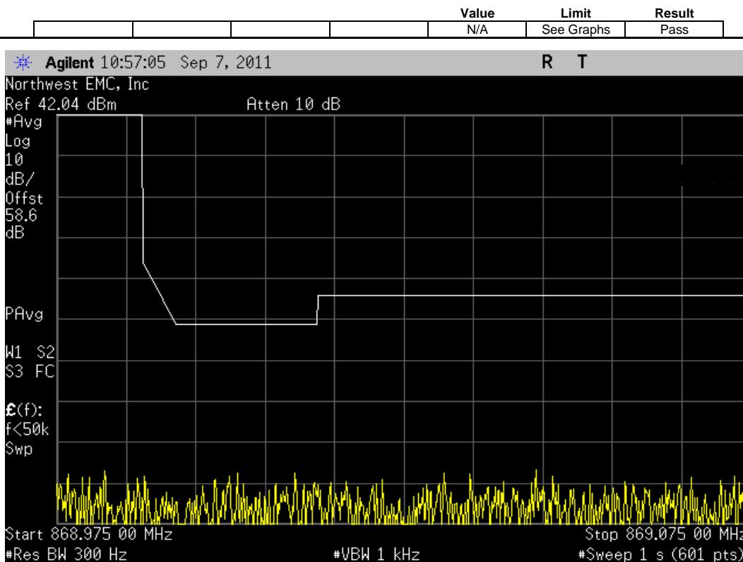
CDMA, Antenna Port B, Multi Carrier [3 FA], (862.9 MHz, 865.4 MHz, 867.9 MHz), Upper Band Edge Zoomed Out
