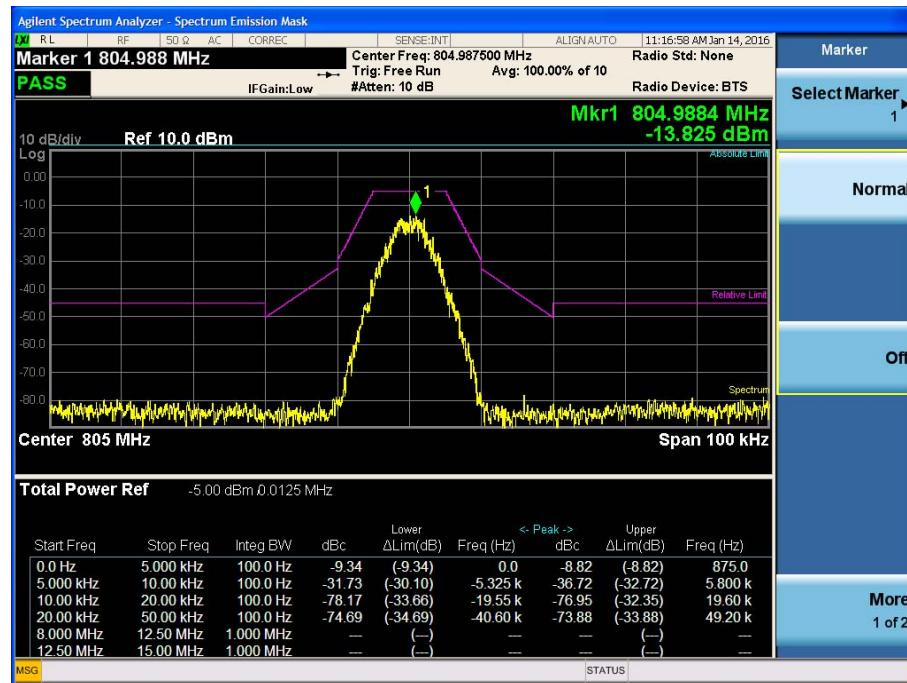
[+3 dB Above the AGC Threshold Uplink Output FM Low Emission Mask C]
