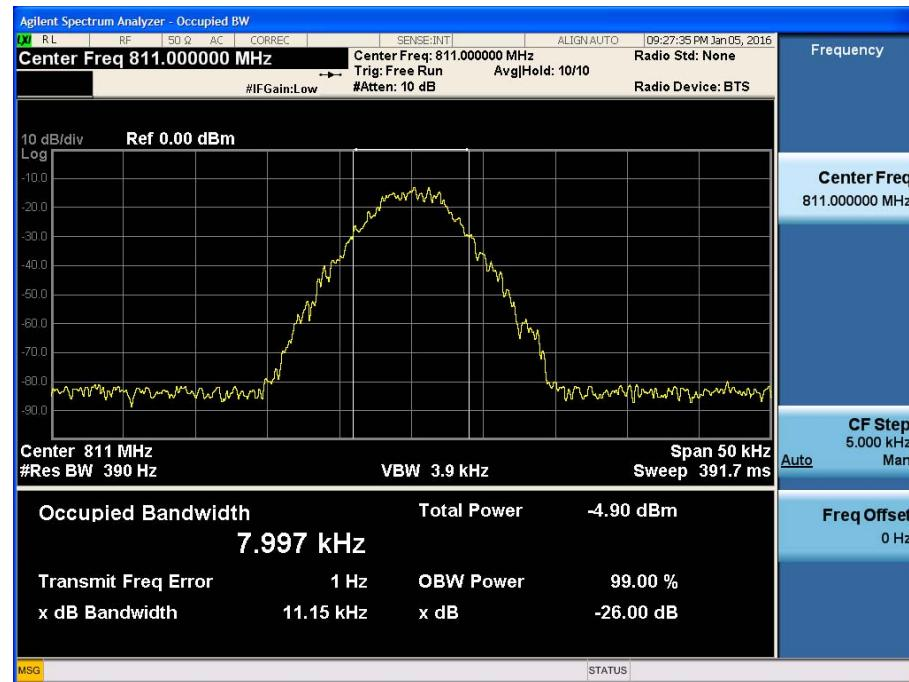
[800 Band +3 dB above the AGC threshold Uplink Output P25 High]
