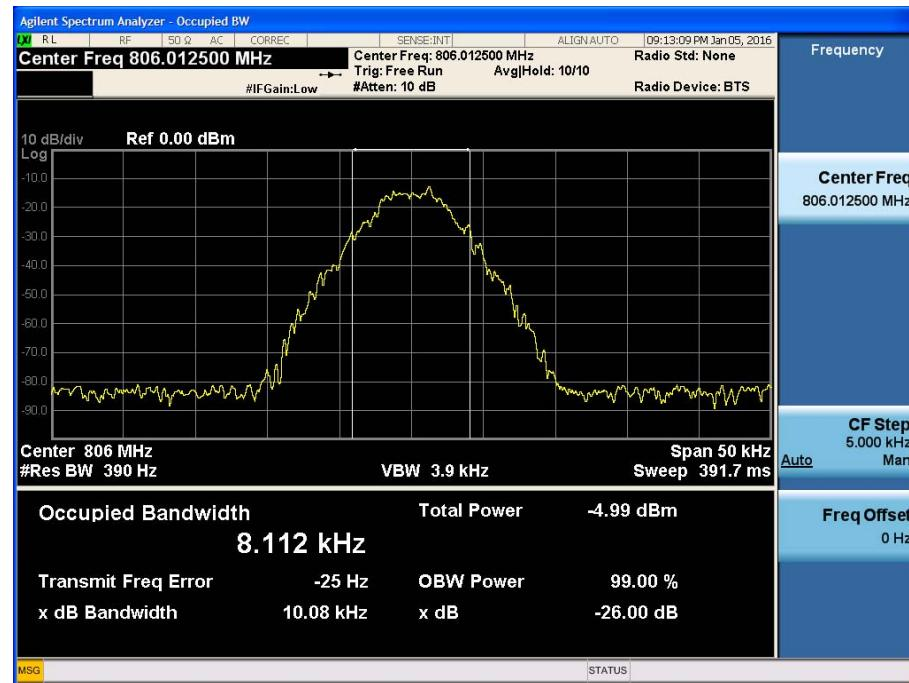
**[800 Band +3 dB above the AGC threshold Uplink Output P25 Middle]**
