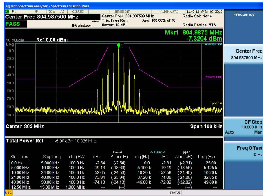
[+3 dB Above the AGC Threshold Uplink Output P25 Low Emission Mask C]
