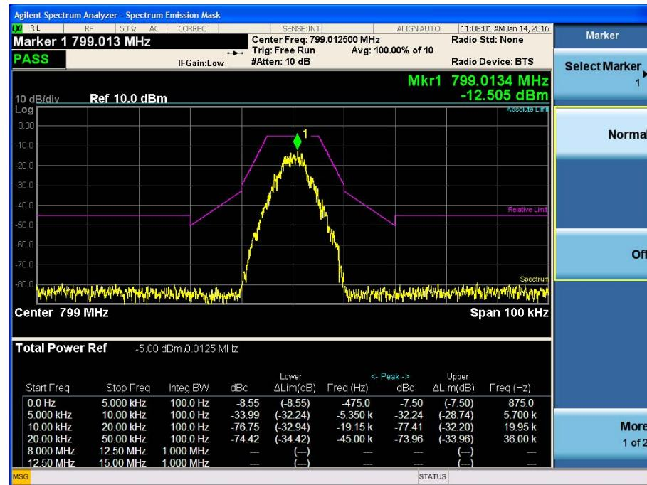
[+3 dB Above the AGC Threshold Uplink Output P25 High Emission Mask C]
