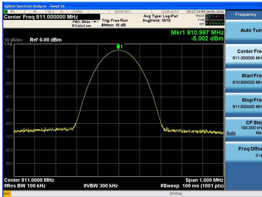
[800 Band +3dB above the AGC threshold Uplink P25 High]
