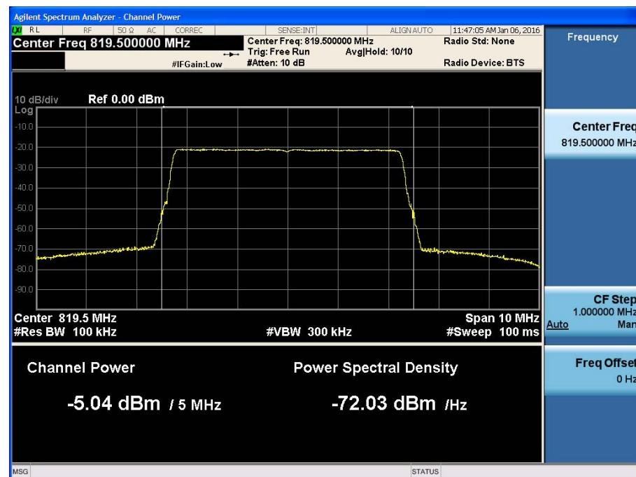
**[800 Band +3dB above the AGC threshold Uplink LTE 5 MHz High]**
