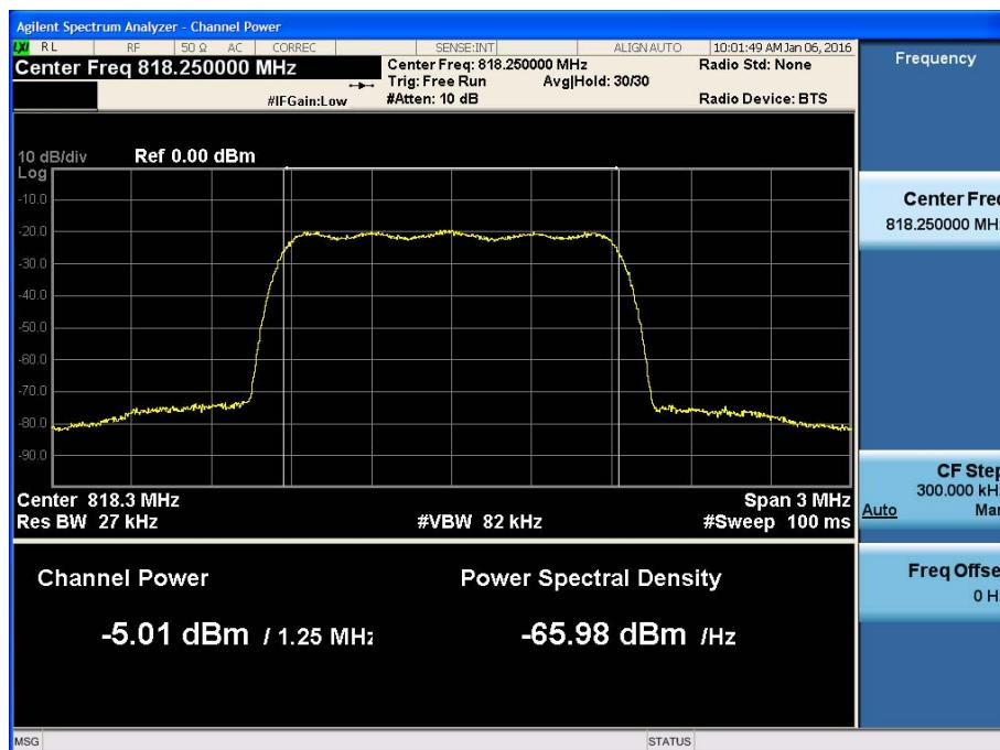
**[800 Band +3dB above the AGC threshold Uplink CDMA 1.25 MHz Middle]**
