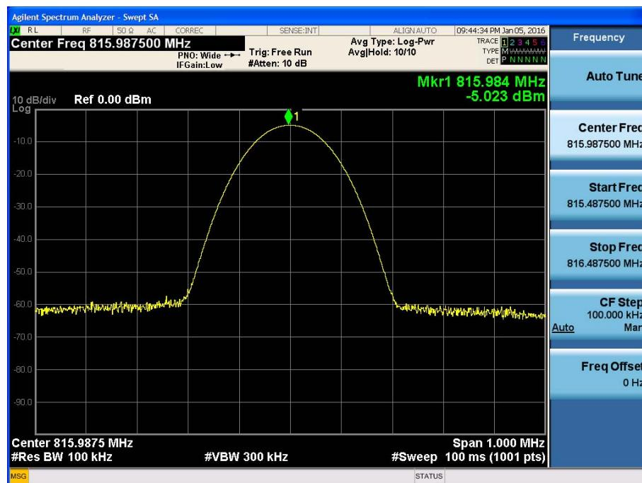
**[800 Band +3dB above the AGC threshold Uplink P25 Low]**
