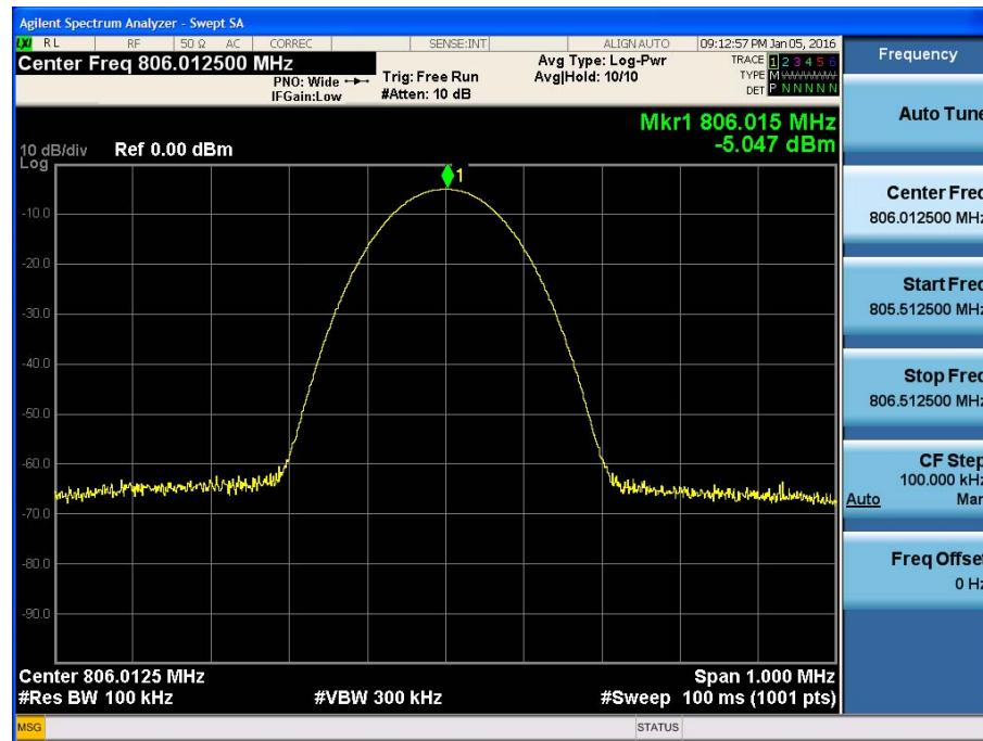
**[800 Band +3dB above the AGC threshold Uplink P25 Middle]**
