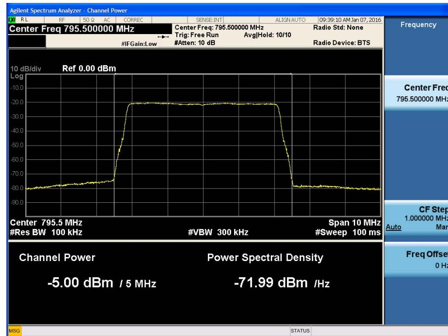
[700 Band +3dB above the AGC threshold Uplink LTE 10 MHz Middle]
