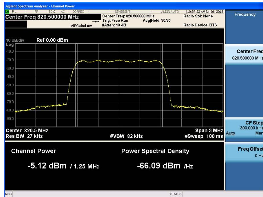
**[800 Band +3dB above the AGC threshold Uplink CDMA 1.25 MHz High]**
