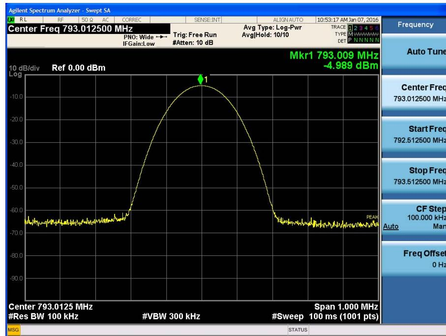
[700 Band +3dB above the AGC threshold Uplink P25 Middle]
