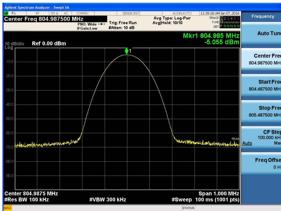
[700 Band +3dB above the AGC threshold Uplink P25 Low]
