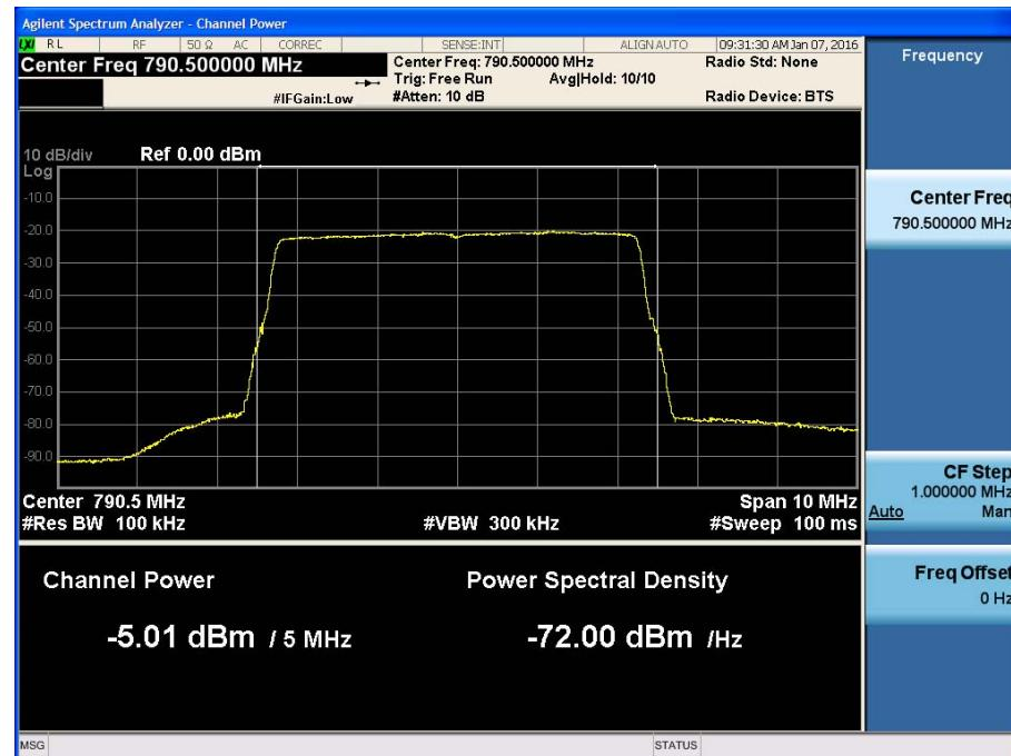
[700 Band +3dB above the AGC threshold Uplink LTE 5 MHz High]
