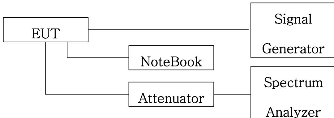
**Block Diagram 1. RF Power Output Test Setup****Test Results:**
