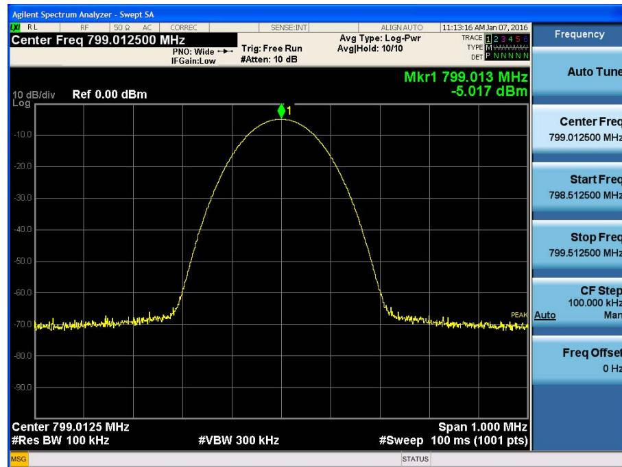
[700 Band +3dB above the AGC threshold Uplink P25 High]
