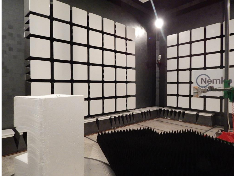
Figure 8.2-4: Emissions setup photo – above 1 GHz
