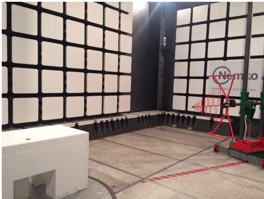
Figure 8.2-3: Emissions setup photo – 30 to 1000 MHz
