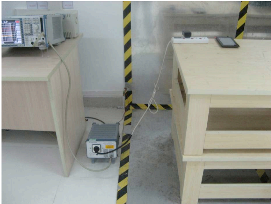
CONDUCTED EMISSION TEST SETUP
