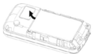
Then gently press the battery downward using the finger, and then press the other end to install the battery.
