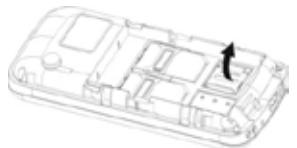
**Prompt: If the memory card is failed, please check whether it is correctly placed and good contact of metal point.**
