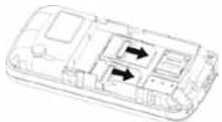
**Prompt: Please make sure to power off the phone before taking out SIM card. It is absolutely forbidden to insert or take out SIM card with external power supply; otherwise it may damage SIM card and the phone.**
