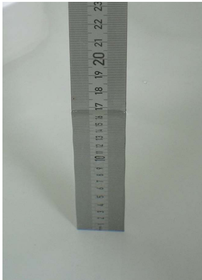
Fig. 17: Liquid depth for IEEE 802.11 b/g body measurements
