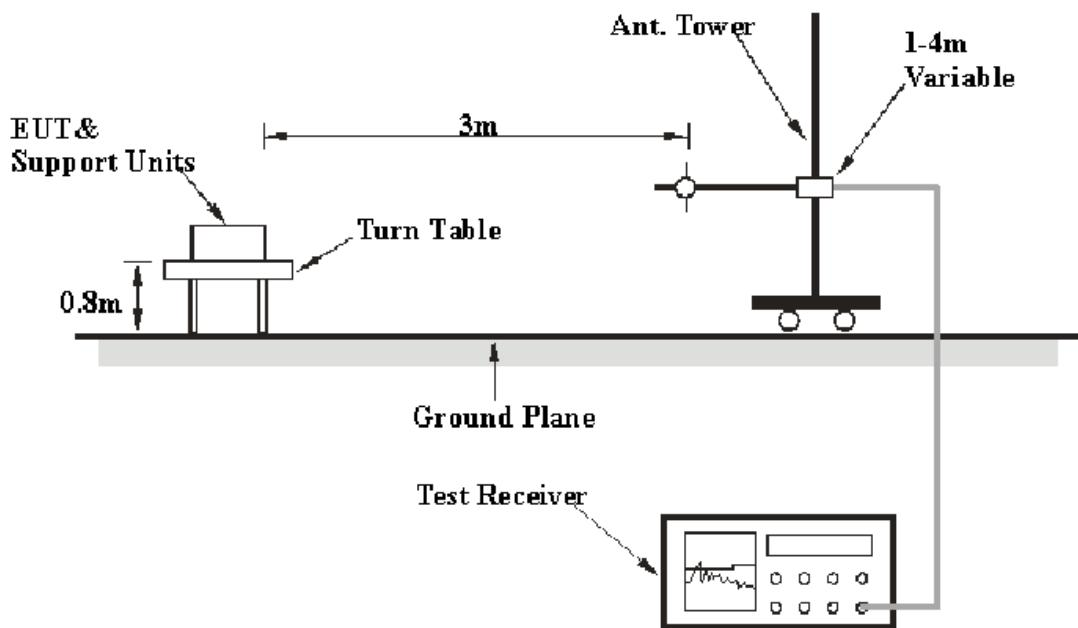
The radiated emission tests were performed in the 3 meters chamber B test site, using the setup accordance with the ANSI C63.17 - 2006. The specification used was the FCC 15§ 15.319(g).
