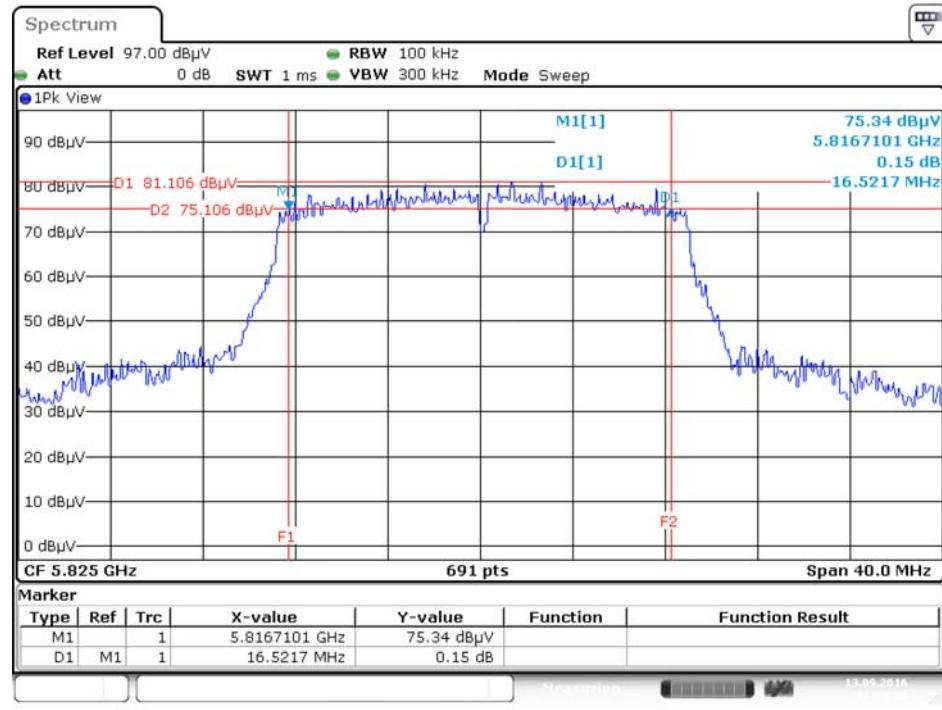
**6 dB Bandwidth Plot on Configuration IEEE 802.11ac MCS0/Nss1 VHT40 / Ant. 1 + Ant. 2 + Ant. 4 / 5755 MHz**
