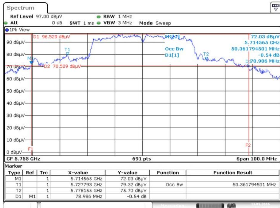
**26dB Bandwidth and 99% Occupied Bandwidth Plot on Configuration IEEE 802.11ac MCS0/Nss1 VHT40 /
