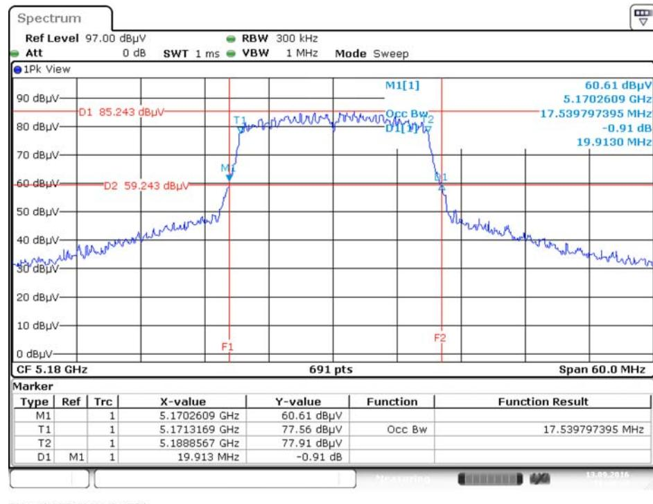
**26dB Bandwidth and 99% Occupied Bandwidth Plot on Configuration IEEE 802.11ac MCS0/Nss1 VHT20 / Ant. 1 + Ant. 2 + Ant. 4 / 5200 MHz**
