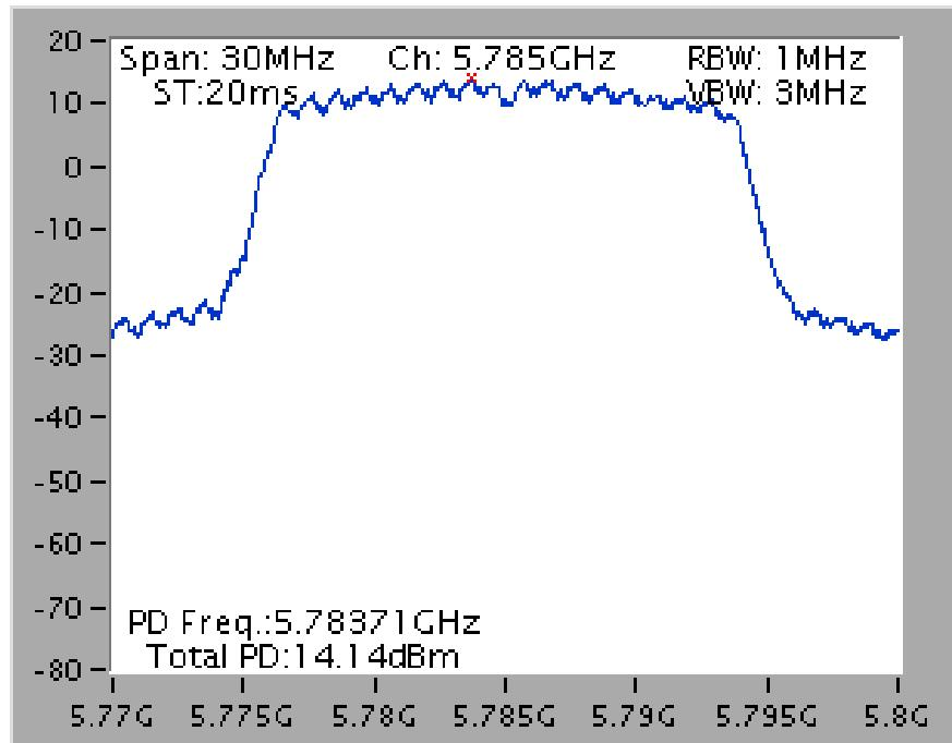
Power Density Plot on Configuration IEEE 802.11ac MCS0/Nss1 VHT20 / Ant. 1 + Ant. 2 + Ant. 4 / 5200 MHz
