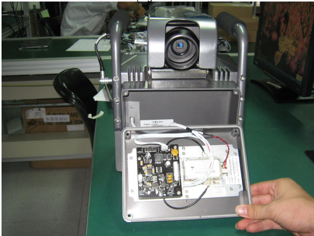
Radar Inside (Right side is Transmitter)
