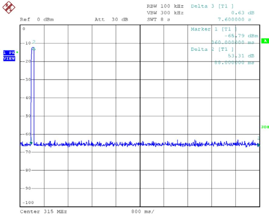
**Note:** “Marker 1” mean the moment button is pressed, and “Marker 2” mean where the button is released (no longer pressed). Then, from the plot, TX must be deactivated within 5 sec.
