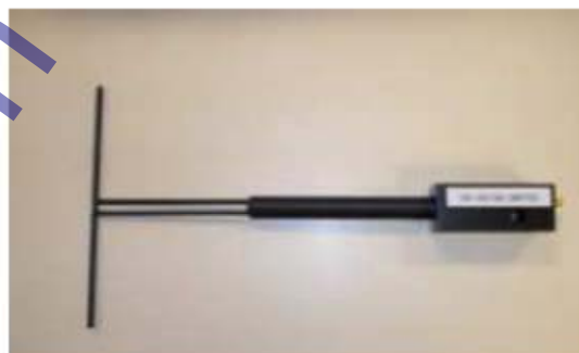
Figure 1 – Satimo COMOSAR Validation Dipole
