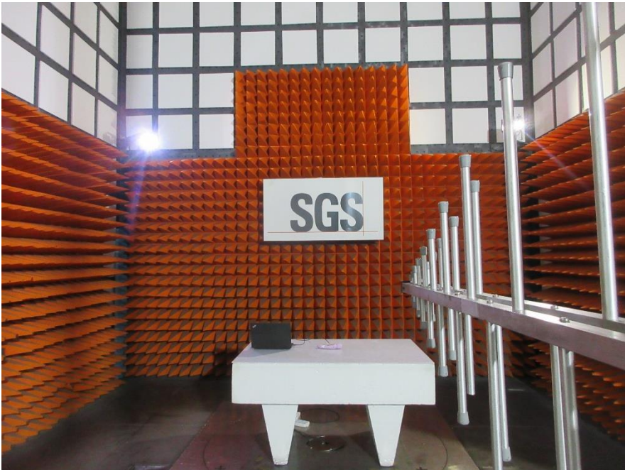
Radiated Spurious Emissions Below 1GHz
