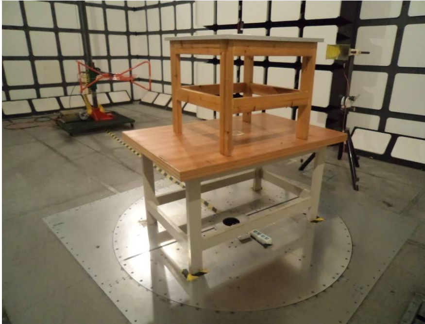
Radiated Emissions Test View (Below 1 GHz)
