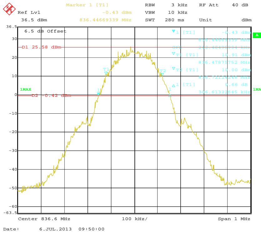
**PCS Band (Part 24E)****99% Occupied Bandwidth & 26 dB Emissions Bandwidth**
