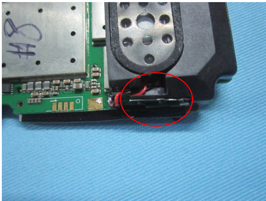
WIFI Antenna View
