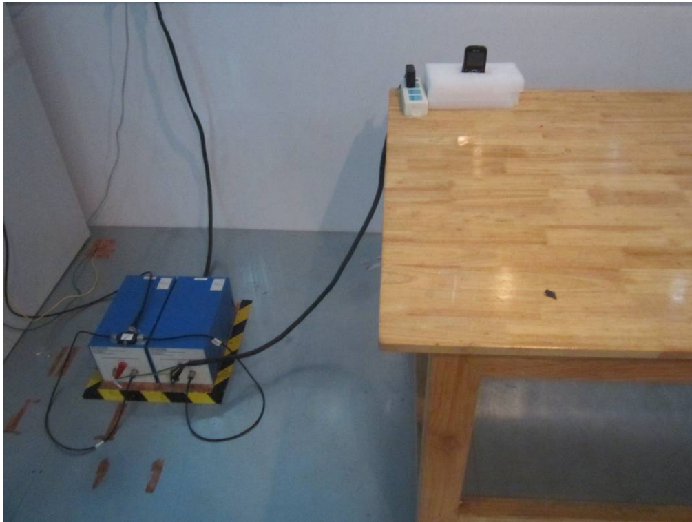
Conducted Emissions Test Setup Front View
