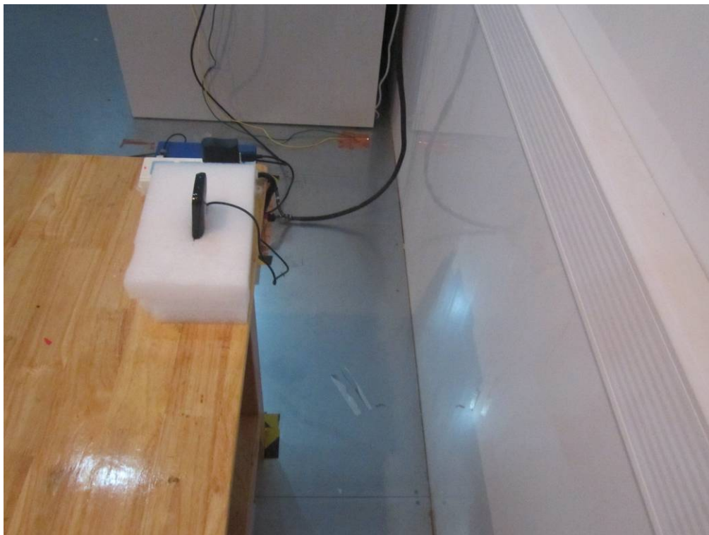
Conducted Emissions Test Setup Side View
