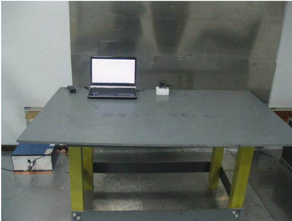
Conducted Emissions Test Setup - Front View
