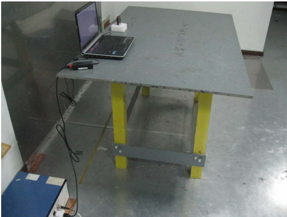
Conducted Emissions Test Setup - Side View
