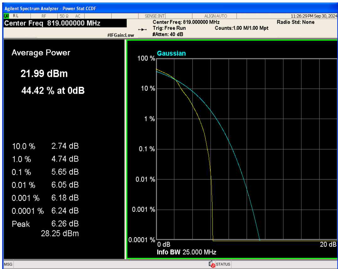
Band26b QPSK BW=1.4MHz Channel=26915 RB Size=1 Position=#0
