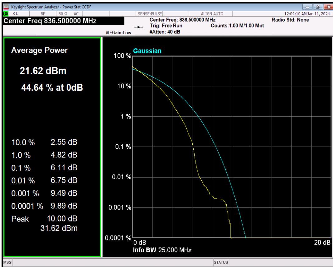
Band5 16QAM BW=5MHz Channel=20525 RB Size=1 Position=#0
