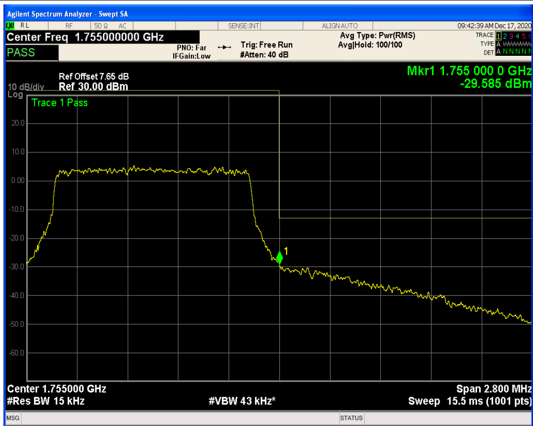
Band4 QPSK BW=3MHz Channel=19965 RB Size=1 Position=#Max
