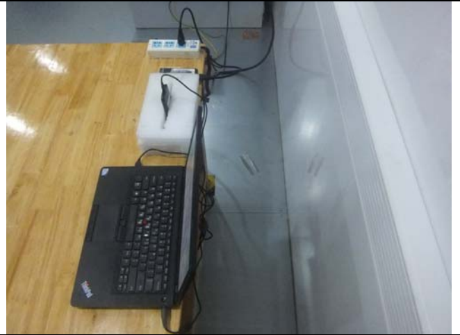
Conducted Emissions Test Setup – Side View
