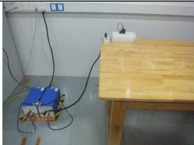
Conducted Emissions Test Setup Front View
