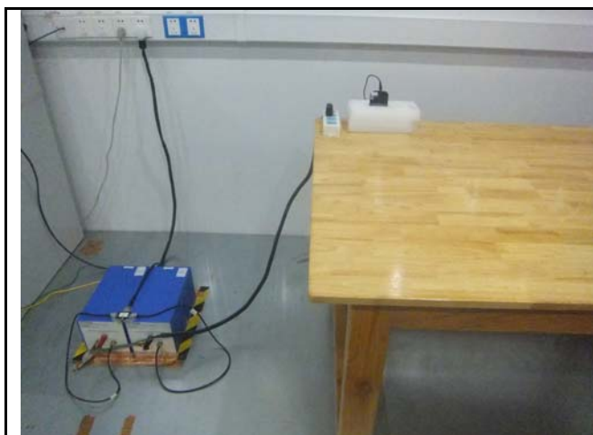
Conducted Emissions Test Setup Front View
