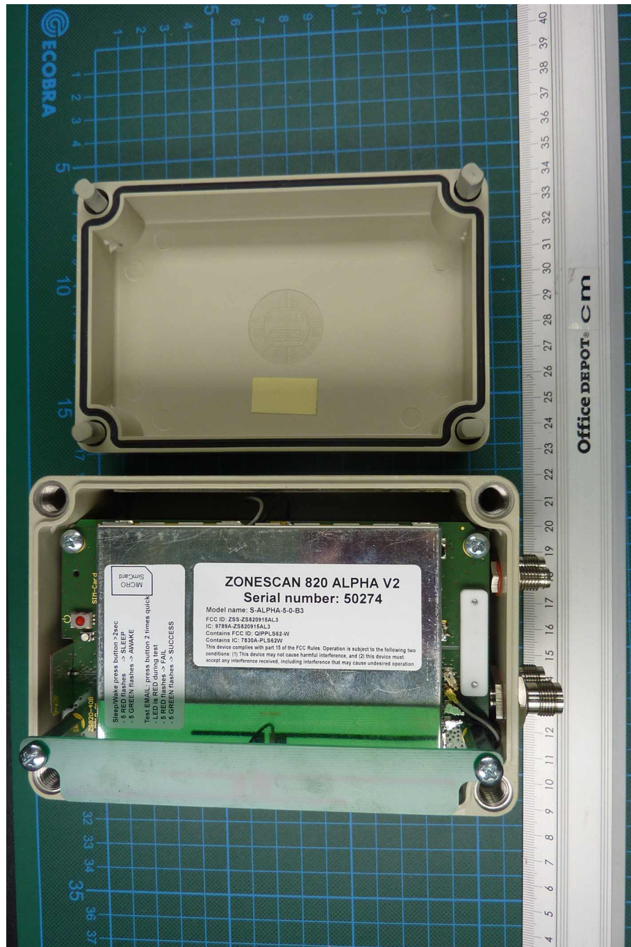
ZONESCAN 820 Alpha V2, internal view (housing opened)
