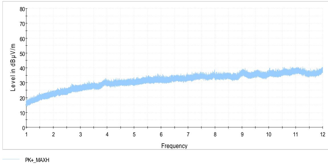
190760\_12G\_14G\_15B: Preliminary emission measurement from 12 GHz to 14 GHz:
