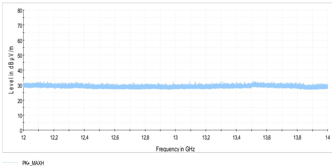
No significant frequencies above the noise floor of the system (max 40.9 dB $\mu$ V/m (measured with peak detector) at 3 m distance) were found during the preliminary radiated emission test, so no final measurements were carried out.
