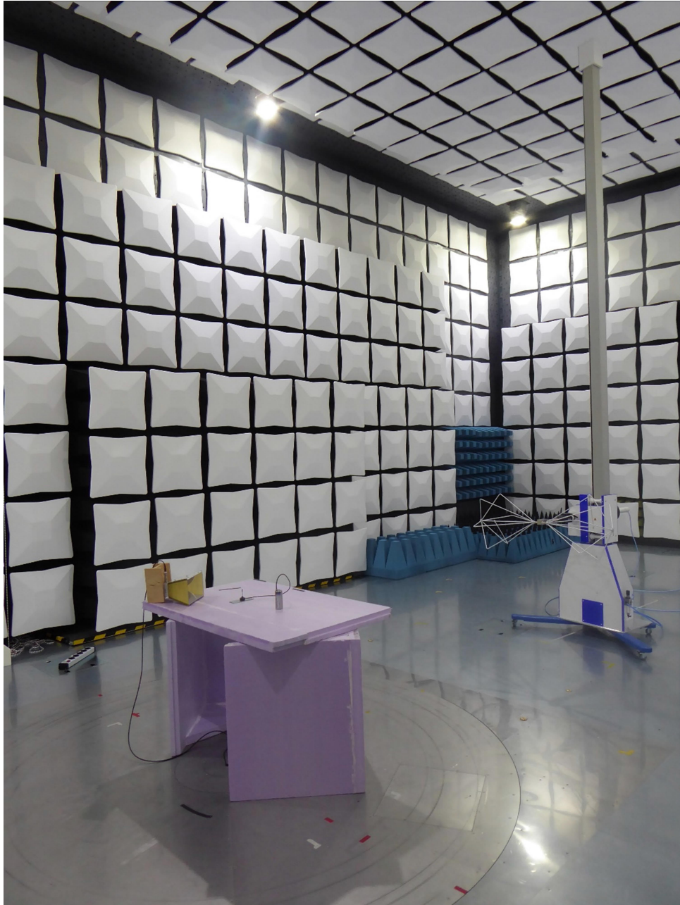
Test Setup SAC from 30 MHz to 200 MHz
