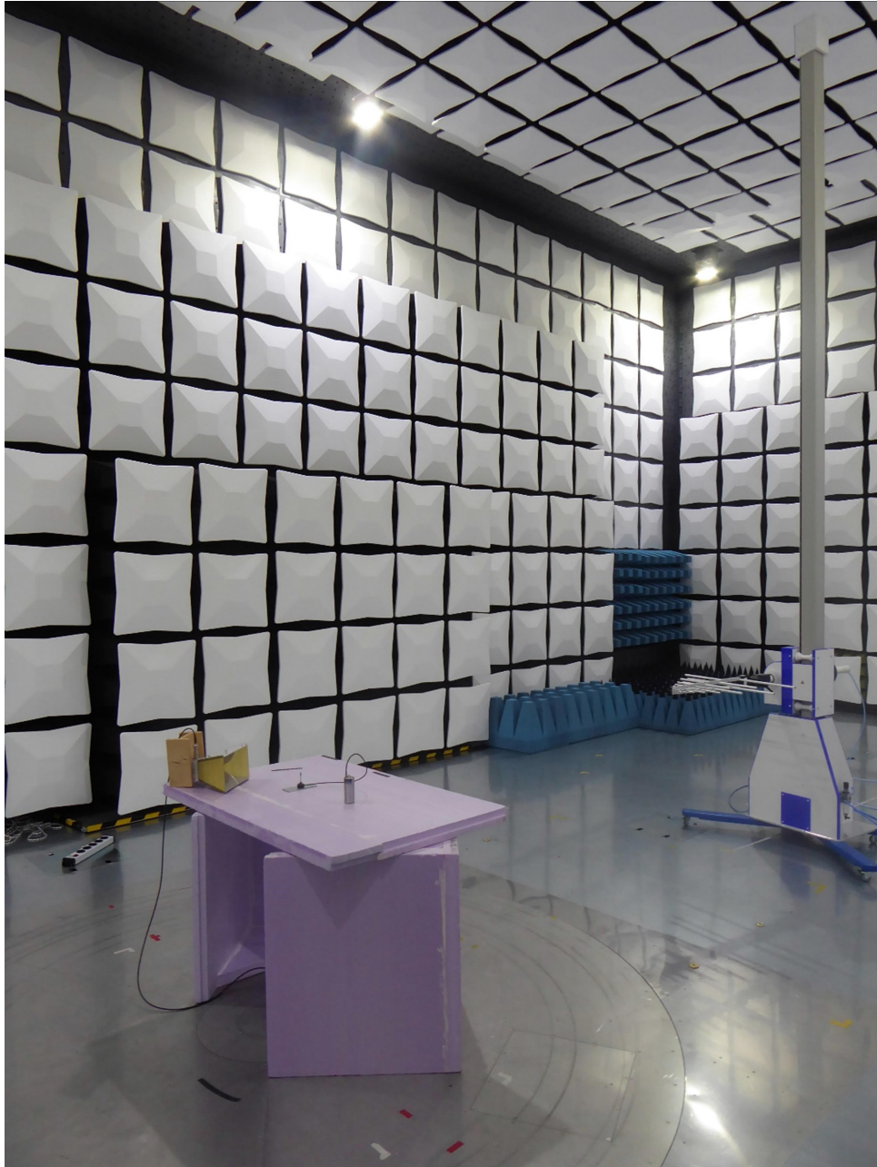
Test Setup SAC from 200 MHz to 1 GHz
