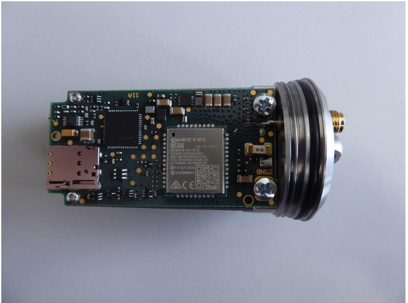
EUT on PCB of IoT Leak Logger (host device), top view
