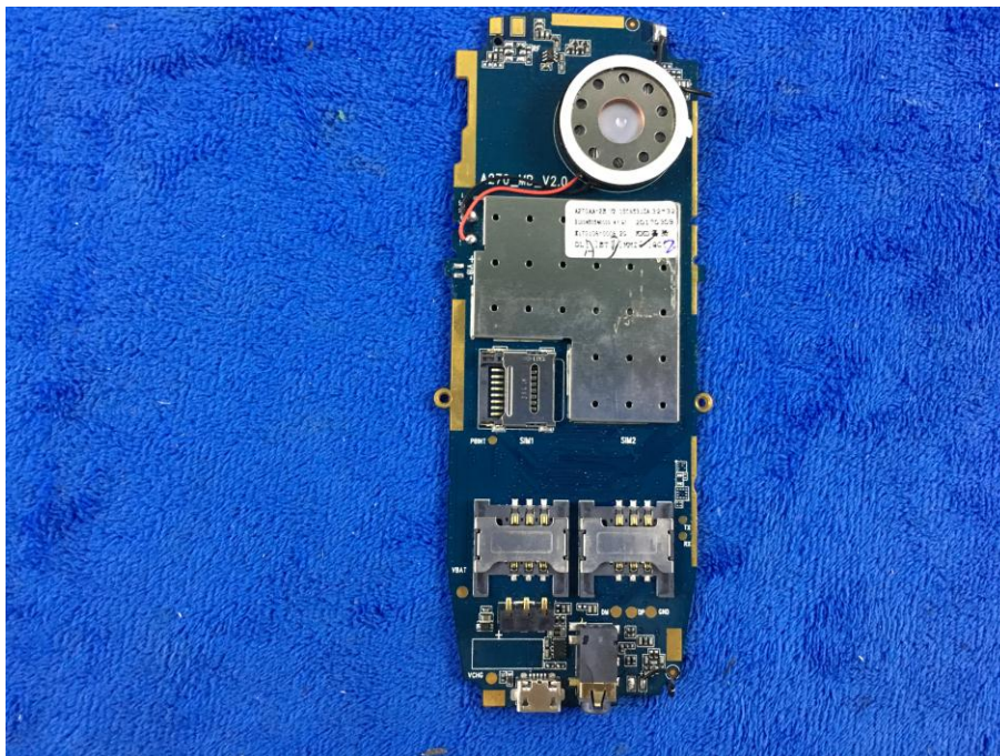
Mainboard with shielding - Rear View
