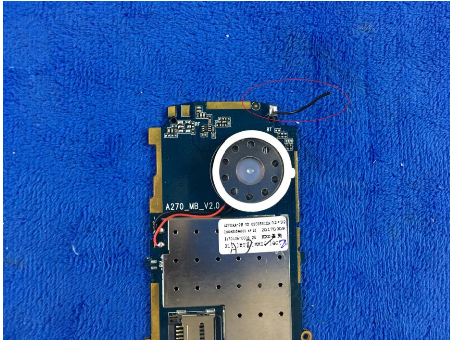
BT - Antenna View
