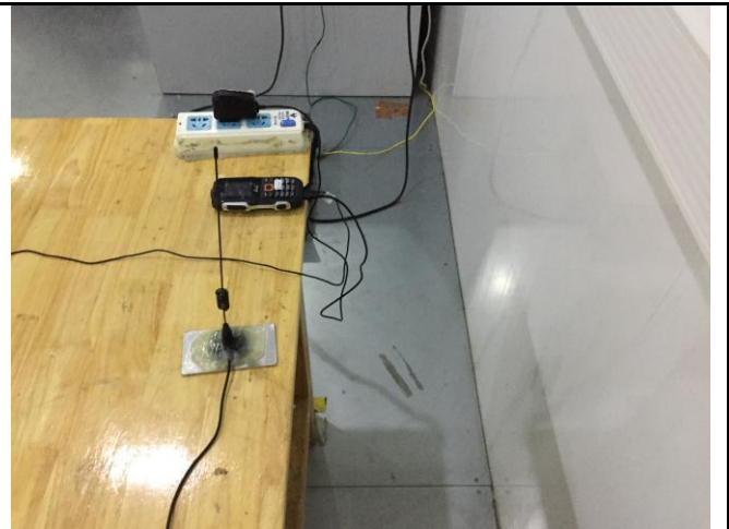
Conducted Emissions Test Setup Side View
