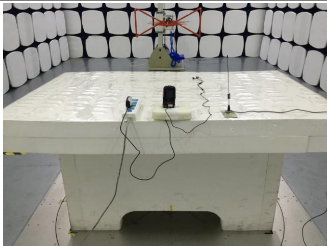
Conducted Emissions Test Setup Front View
