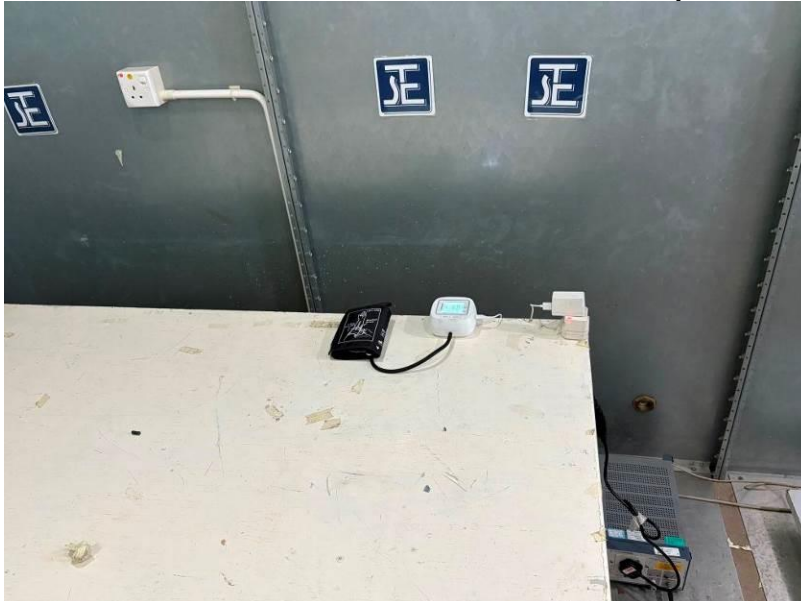
Measurement of Conducted Emission Test Set Up
