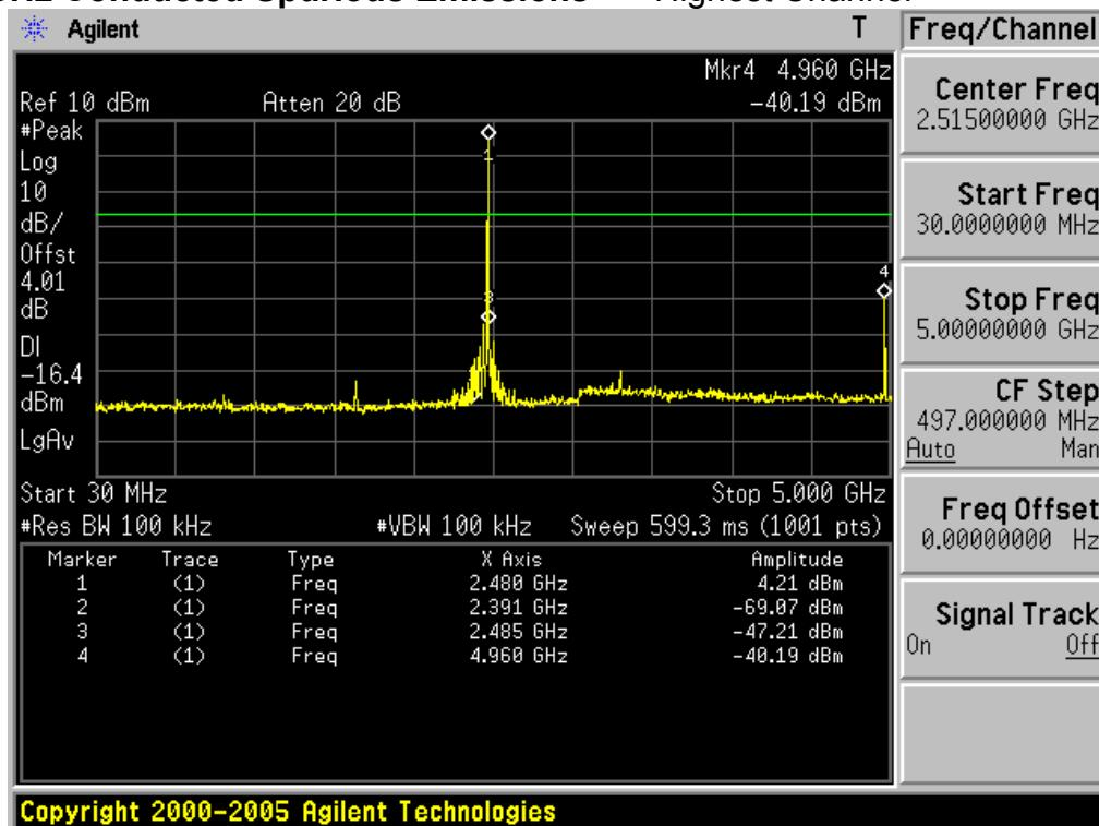
**5GHz ~ 10GHz Conducted Spurious Emissions      Highest Channel**
