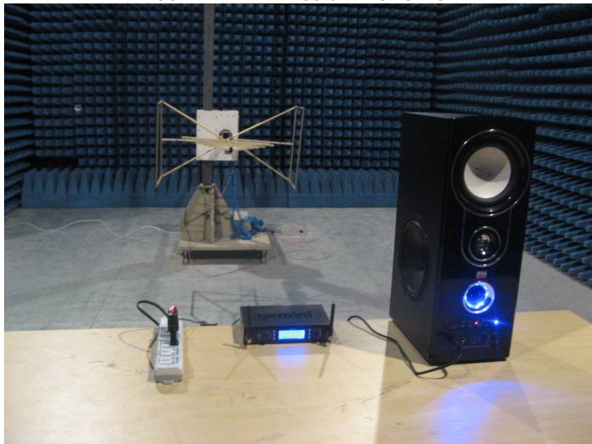
FCC RADIATED EMISSION TEST SETUP
